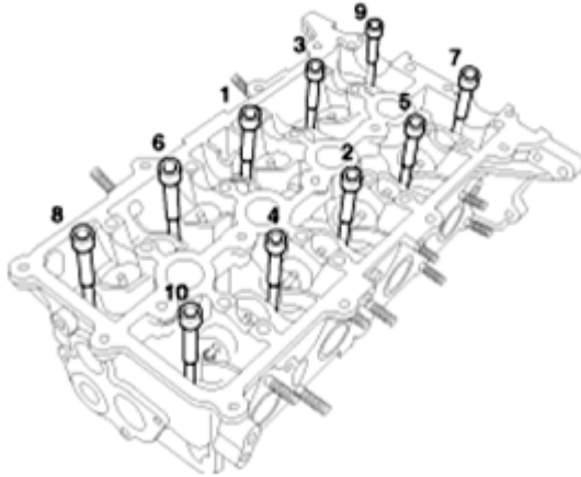
Fig. 23: Identifying Tightening Sequence Of Cylinder Head Bolts Courtesy of KIA MOTORS AMERICA, INC.
