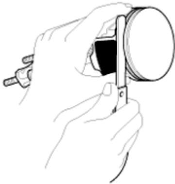
Fig. 24: Measuring Clearance Between Piston Ring & Wall Of Ring Groove Courtesy of KIA MOTORS AMERICA, INC.
