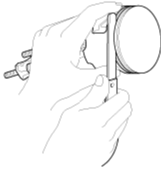
Fig. 28: Measuring Clearance Between Piston Ring And Wall Of Ring Groove Courtesy of KIA MOTORS AMERICA, INC.
