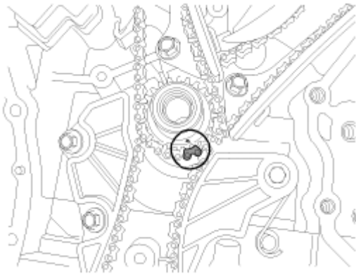
Fig. 46: Identifying Timing Mark Of Timing Chain Courtesy of KIA MOTORS AMERICA, INC.
