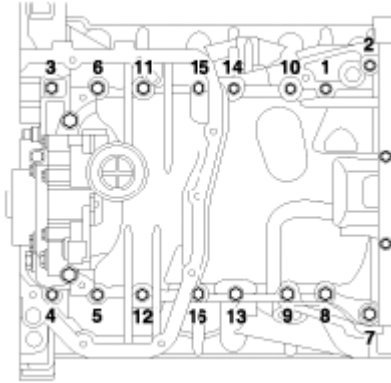
Fig. 48: Identifying Oil Pan Bolts In Tightening Sequence Courtesy of KIA MOTORS AMERICA, INC.
