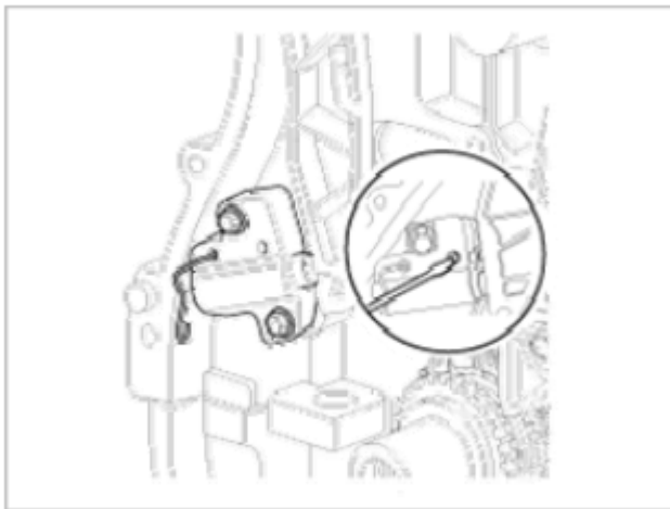
Fig. 55: Installing Set Pin
