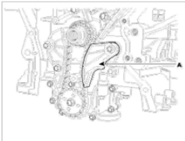
Fig. 59: Identifying Oil Pump Chain Tensioner Assembly
