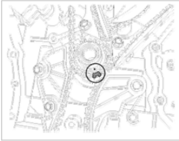
Fig. 79: Identifying Timing Mark On Crankshaft Sprocket
