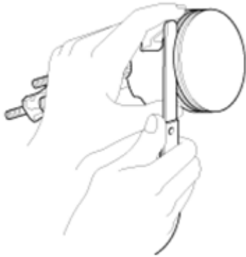
Fig. 30: Measuring Piston Ring Side Clearance
