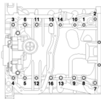
Fig. 50: Upper Oil Pan Bolts Tightening Sequence Courtesy of KIA MOTORS AMERICA, INC.
