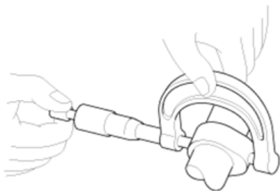
Fig. 21: Measuring Cam Lobe Height Courtesy of KIA MOTORS AMERICA, INC.
