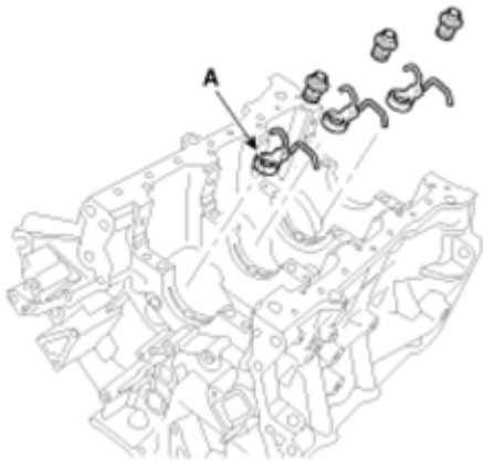
Fig. 36: Oil Jets Courtesy of KIA MOTORS AMERICA, INC.
