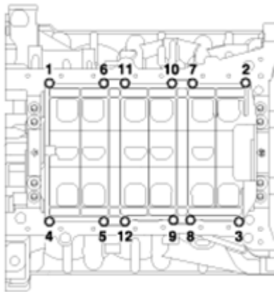
Fig. 46: Identifying Baffle Plate Bolts Tightening Sequence Courtesy of KIA MOTORS AMERICA, INC.
