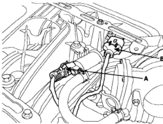
Fig. 40: Locating PCSV Connector, MAP Sensor Connector And PCSV Hose Courtesy of KIA MOTORS AMERICA, INC.
