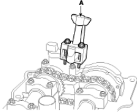
Fig. 52: Identifying Timing Chain Auto Tensioner Courtesy of KIA MOTORS AMERICA, INC.
