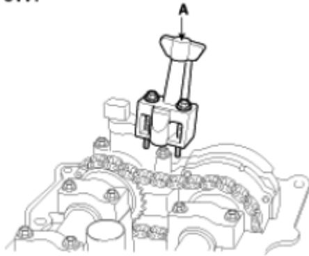
Fig. 17: Identifying Timing Chain Auto Tensioner Courtesy of KIA MOTORS AMERICA, INC.
