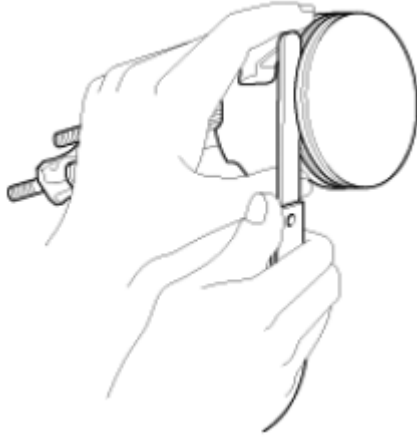
Fig. 26: Measuring Clearance Between Piston Ring And Wall Of Ring Groove Using Feeler Gauge Courtesy of KIA MOTORS AMERICA, INC.
