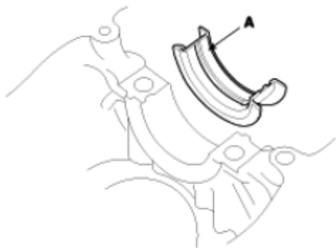
Fig. 35: Identifying Center Bearing Courtesy of KIA MOTORS AMERICA, INC.
