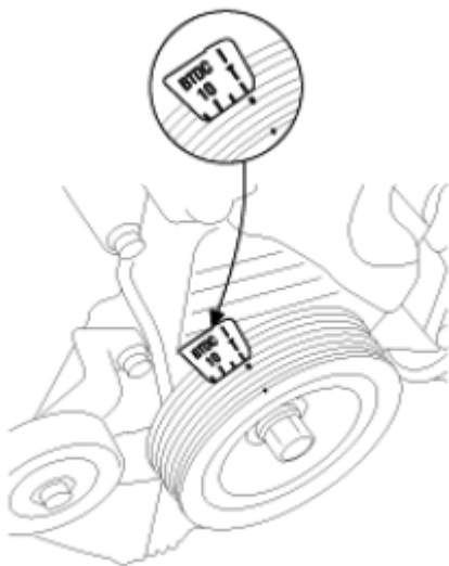
Fig. 8: Aligning Crankshaft Pulley Groove With Timing Mark "T" Of Timing Belt Cover Courtesy of KIA MOTORS AMERICA, INC.
