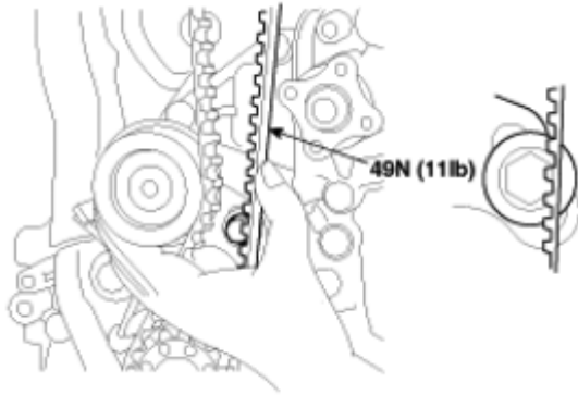
Fig. 14: Checking Belt Tension Courtesy of KIA MOTORS AMERICA, INC.
