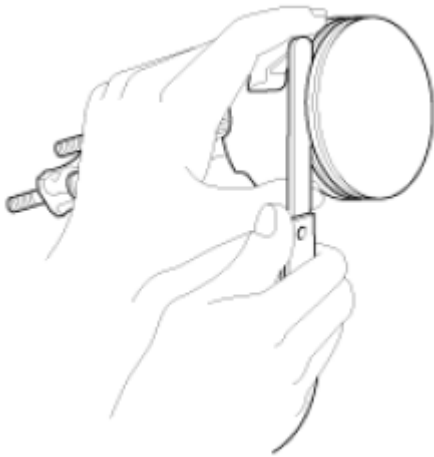
Fig. 31: Measuring Piston Outside Diameter From Bottom Of Piston Courtesy of KIA MOTORS AMERICA, INC.
