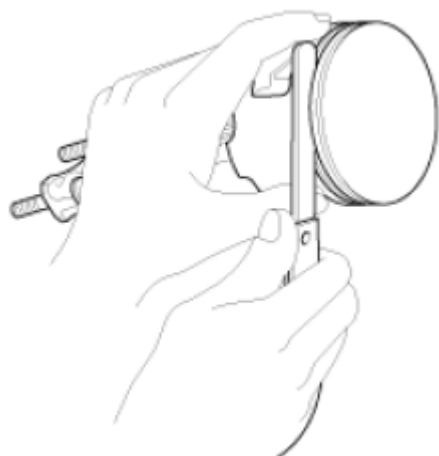
Fig. 32: Measuring Clearance Between Piston Ring And Ring Groove Courtesy of KIA MOTORS AMERICA, INC.
