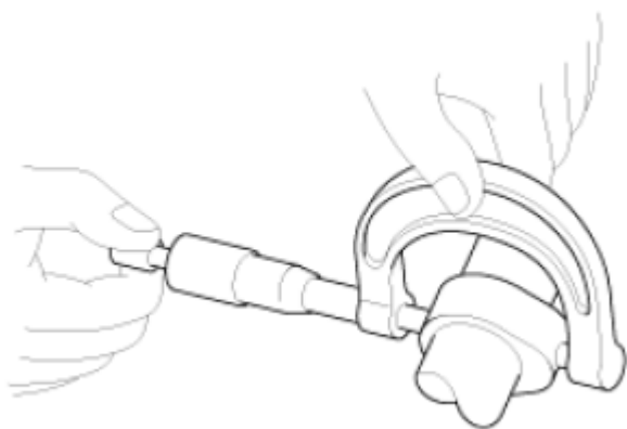
Fig. 38: Measuring Cam Lobe Height Courtesy of KIA MOTORS AMERICA, INC.
