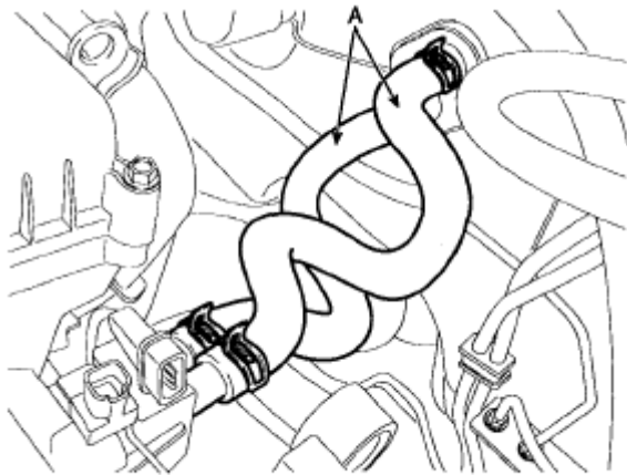
Fig. 125: Identifying Heater Hoses Courtesy of KIA MOTORS AMERICA, INC.
