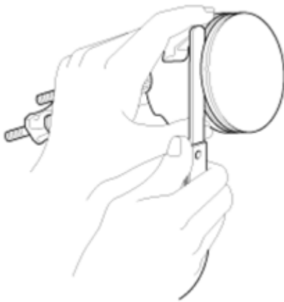
Fig. 29: Measuring Piston Ring Side Clearance Courtesy of KIA MOTORS AMERICA, INC.
