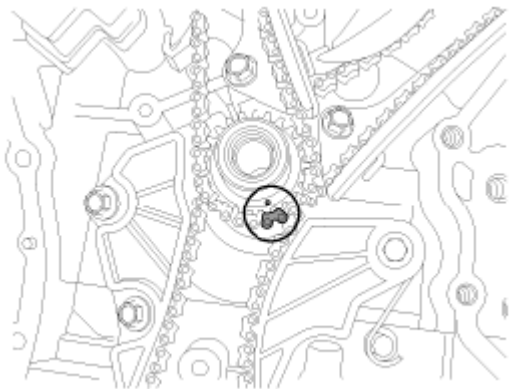
Fig. 68: Identifying Timing Mark Of Timing Chain Courtesy of KIA MOTORS AMERICA, INC.
