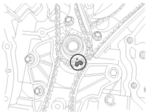
Fig. 41: Identifying Marks On Sprockets & RH/LH Timing Chain (2 Of 4) Courtesy of KIA MOTORS AMERICA, INC.
