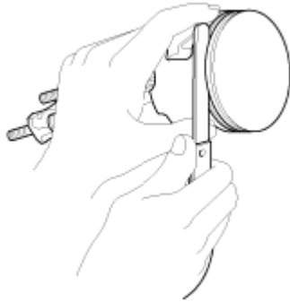
Fig. 30: Measuring Clearance Between Piston Ring & Wall Of Ring Groove Courtesy of KIA MOTORS AMERICA, INC.
