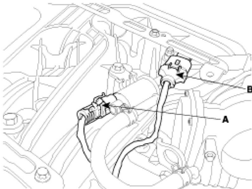
Fig. 136: Identifying PCSV Connector & MAP Sensor Connector Courtesy of KIA MOTORS AMERICA, INC.
