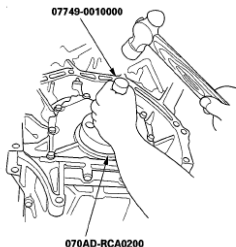
Fig. 71: Installing Crankshaft Oil Seal
