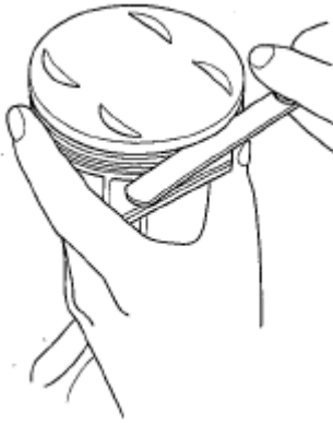
Fig. 47: Measuring Ring-To-Groove Clearance: Courtesy of AMERICAN HONDA MOTOR CO., INC.
