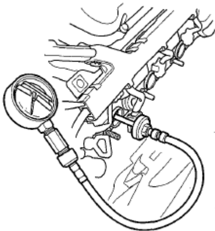
Fig. 6: Attaching Compression Gauge To Spark Plug Hole Courtesy of AMERICAN HONDA MOTOR CO., INC.
