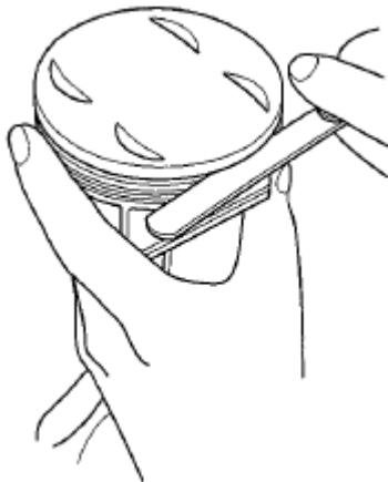
Fig. 48: Measuring Ring-To-Groove Clearance
