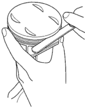
Fig. 52: Measuring Ring-To-Groove Clearance
