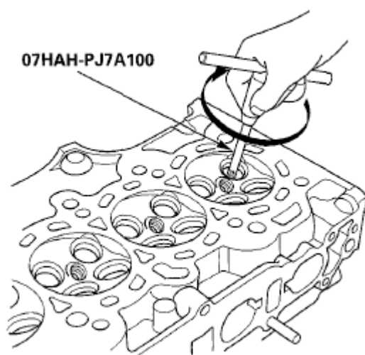
Fig. 108: Rotating Reamer Of Valve Guide Bore Courtesy of AMERICAN HONDA MOTOR CO., INC.
