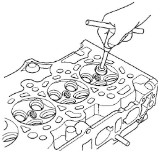
Fig. 109: Reconditioning Valve Seats In Cylinder Head Courtesy of AMERICAN HONDA MOTOR CO., INC.
