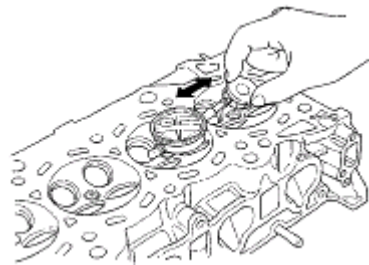
Fig. 110: Measuring Valve Stem-To-Guide Clearance
