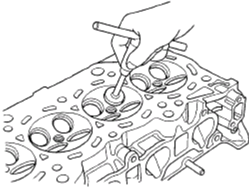
Fig. 116: Reaming Valve Seats In Cylinder Head Courtesy of AMERICAN HONDA MOTOR CO., INC.
