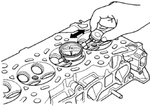
Fig. 119: Measuring Stem-To-Guide Clearance With Dial Indicator Courtesy of AMERICAN HONDA MOTOR CO., INC.
