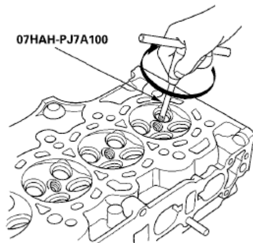
Fig. 115: Installing Valve Guide Seal Remover
