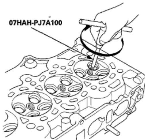
Fig. 117: Rotating Reamer Clockwise Full Length Of Valve Guide Bore Courtesy of AMERICAN HONDA MOTOR CO., INC.
