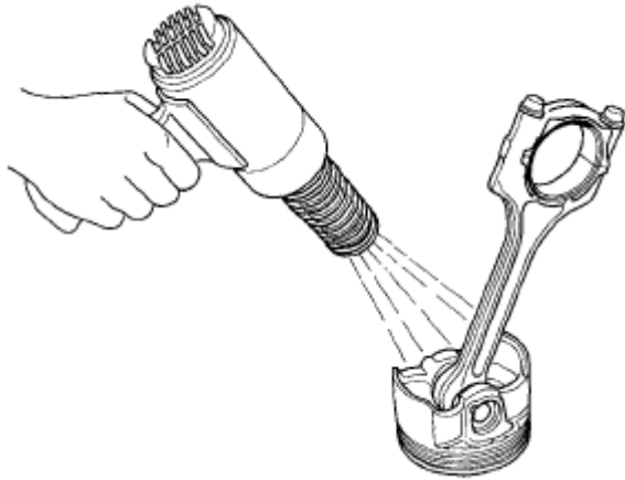
Fig. 35: Heating Piston And Connecting Rod Assembly Courtesy of AMERICAN HONDA MOTOR CO., INC.
