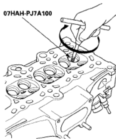
Fig. 116: Rotating Reamer To Valve Guide Bore Courtesy of AMERICAN HONDA MOTOR CO., INC.
