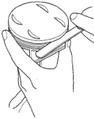
Fig. 48: Measuring Ring-To-Groove Clearance
