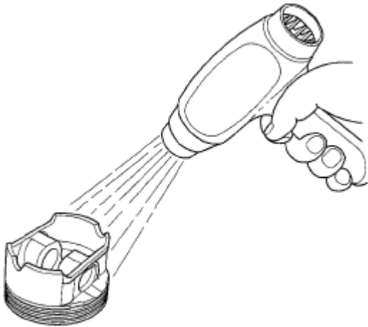
Fig. 43: Heating Piston To About 158°F (70°C)
