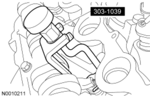
Fig. 138: Identifying Special Tool (303-1039) For Removing/Installing Camshaft Roller Followers Courtesy of FORD MOTOR CO.
