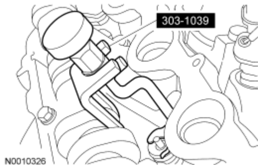
Fig. 388: Compressing Valve Spring With Special Tool (303-1039) Courtesy of FORD MOTOR CO.
