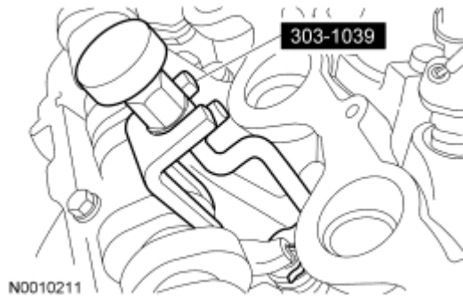
Fig. 147: Identifying Special Tool (303-1039) For Removing/Installing Camshaft Roller Followers Courtesy of FORD MOTOR CO.
