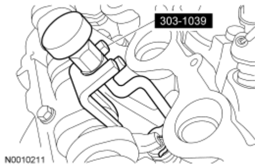
Fig. 151: Identifying Special Tool (303-1039) For Removing/Installing Camshaft Roller Followers Courtesy of FORD MOTOR CO.
