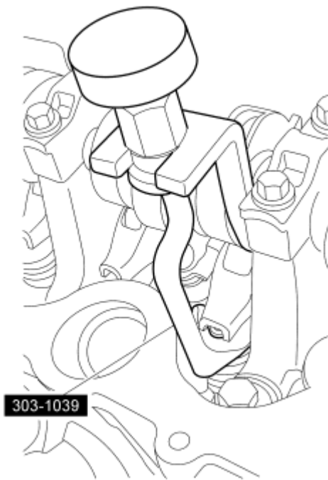
Fig. 290: Compressing Spring Using Special Tool (303-1039) Courtesy of FORD MOTOR CO.
