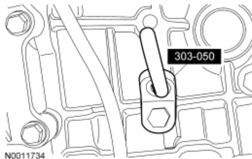
Fig. 242: Installing Special Tool (303-050) To Threaded Hole Located At LH Side Of Engine Block Courtesy of FORD MOTOR CO.
