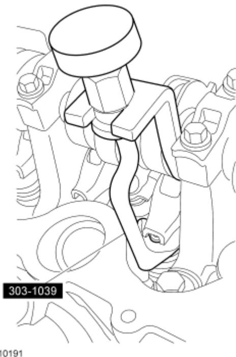
Fig. 115: Compressing Spring Using Special Tool (303-1039) Courtesy of FORD MOTOR CO.
