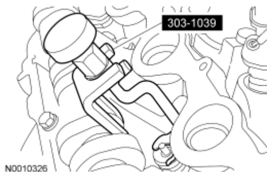
Fig. 150: Compressing Valve Spring With Special Tool (303-1039) Courtesy of FORD MOTOR CO.
