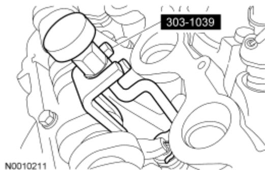
Fig. 288: Identifying Special Tool (303-1039) For Removing/Installing Camshaft Roller Followers Courtesy of FORD MOTOR CO.
