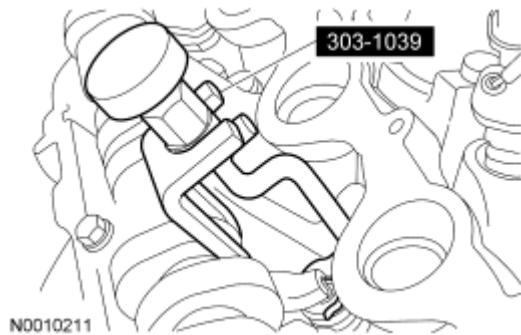
Fig. 152: Identifying Special Tool (303-1039) For Removing/Installing Camshaft Roller Followers Courtesy of FORD MOTOR CO.
