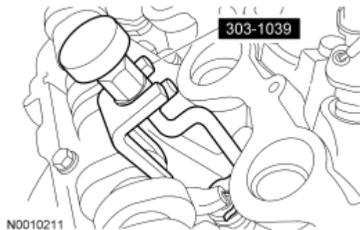
Fig. 146: Identifying Special Tool (303-1039) For Removing/Installing Camshaft Roller Followers Courtesy of FORD MOTOR CO.
