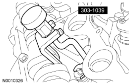
Fig. 149: Compressing Valve Spring With Special Tool (303-1039) Courtesy of FORD MOTOR CO.
