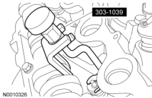
Fig. 392: Compressing Valve Spring With Special Tool (303-1039) Courtesy of FORD MOTOR CO.
