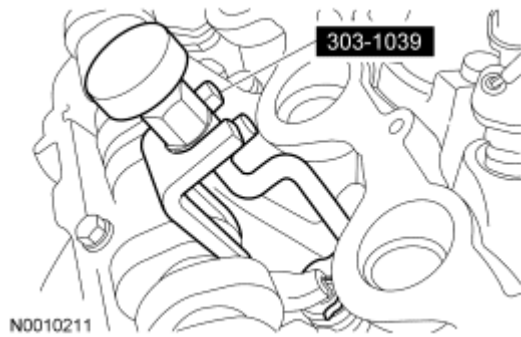
Fig. 58: Identifying Special Tool (303-1039) For Removing/Installing Camshaft Roller Followers Courtesy of FORD MOTOR CO.
