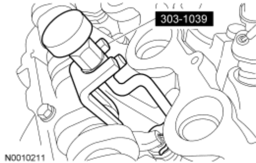
Fig. 124: Identifying Special Tool (303-1039) For Removing/Installing Camshaft Roller Followers Courtesy of FORD MOTOR CO.
