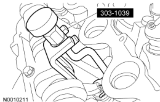
Fig. 148: Identifying Special Tool (303-1039) For Removing/Installing Camshaft Roller Followers Courtesy of FORD MOTOR CO.
