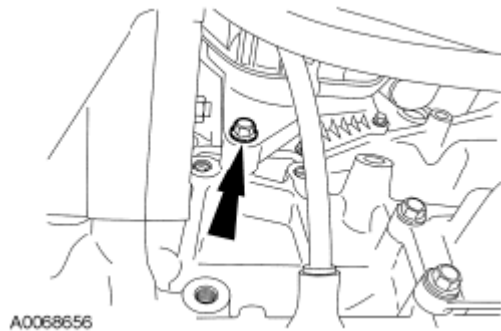
Fig. 209: Identifying Lower Intake Manifold Bolt Courtesy of FORD MOTOR CO.
