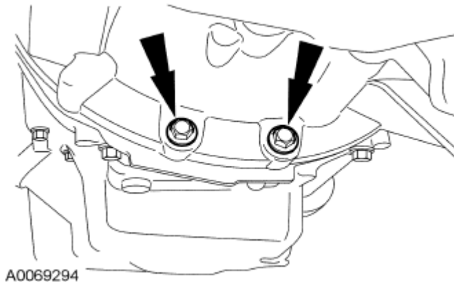
Fig. 407: Locating Lower Bellhousing-To-Oil Pan Bolts Courtesy of FORD MOTOR CO.
