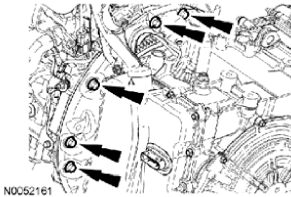
Fig. 117: Identifying Oil Pump Assembly Bolts Tightening Sequence Courtesy of FORD MOTOR CO.
