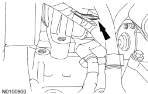
Fig. 17: Locating Engine Wiring Harness Pin-Type Retainer From Intake Manifold Courtesy of FORD MOTOR CO.
