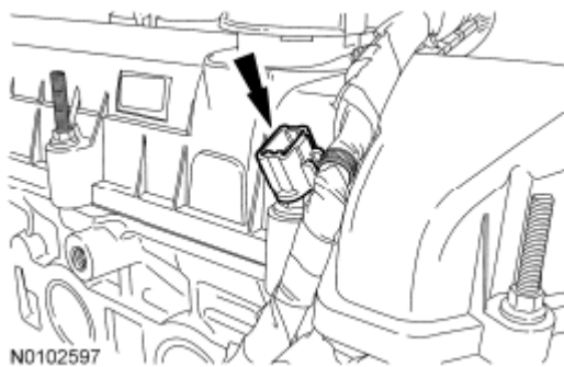
Fig. 367: Locating Wiring Harness Retainer On Valve Cover Stud Courtesy of FORD MOTOR CO.
