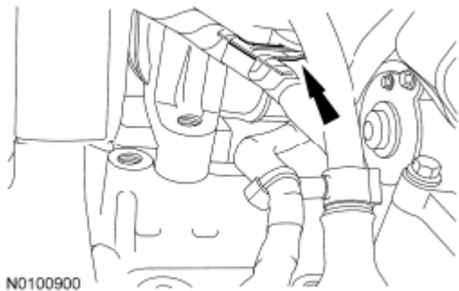
Fig. 9: Locating Engine Wiring Harness Pin-Type Retainer From Intake Manifold Courtesy of FORD MOTOR CO.
