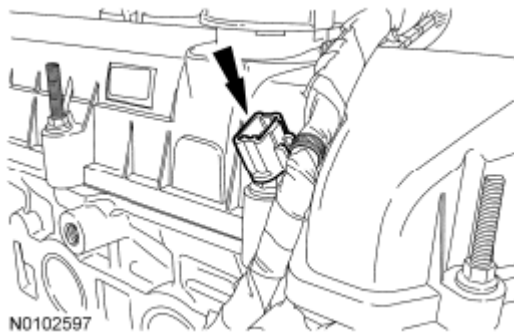
Fig. 202: Locating Generator Wiring Harness Retainer From Valve Cover Stud Courtesy of FORD MOTOR CO.
