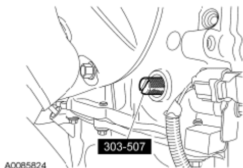
Fig. 104: Removing Crankshaft TDC Timing Peg Courtesy of FORD MOTOR CO.
