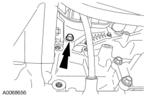
Fig. 231: Locating Lower Intake Manifold Bolt Courtesy of FORD MOTOR CO.
