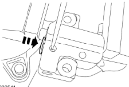
Fig. 77: Pushing Ratchet Arm Back Into Tensioner Housing Courtesy of FORD MOTOR CO.
