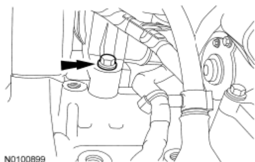
Fig. 8: Locating Intake Manifold Lower Bolt Courtesy of FORD MOTOR CO.
