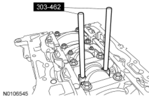
Fig. 274: Removing Piston And Rod Assembly Courtesy of FORD MOTOR CO.
