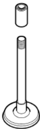
Fig. 113: Identifying Valve Stem Seal Installation Sleeve Courtesy of FORD MOTOR CO.
