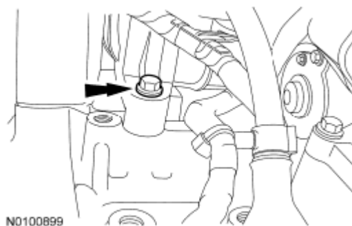
Fig. 18: Locating Lower Intake Manifold Bolt Courtesy of FORD MOTOR CO.
