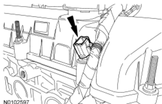
Fig. 385: Locating Generator Wiring Harness Retainer From Valve Cover Stud Courtesy of FORD MOTOR CO.
