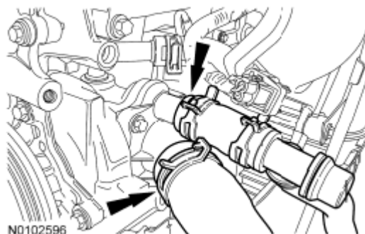
Fig. 229: Locating Wiring Harness Retainers From Intake Manifold Courtesy of FORD MOTOR CO.
