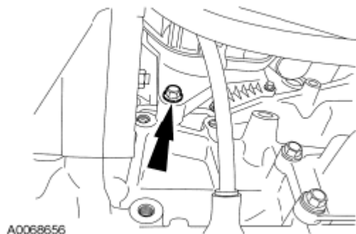
Fig. 377: Locating Lower Intake Manifold Bolt Courtesy of FORD MOTOR CO.
