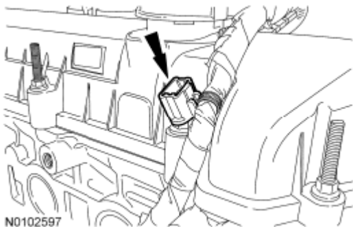
Fig. 224: Locating Generator Wiring Harness Retainer From Valve Cover Stud Courtesy of FORD MOTOR CO.
