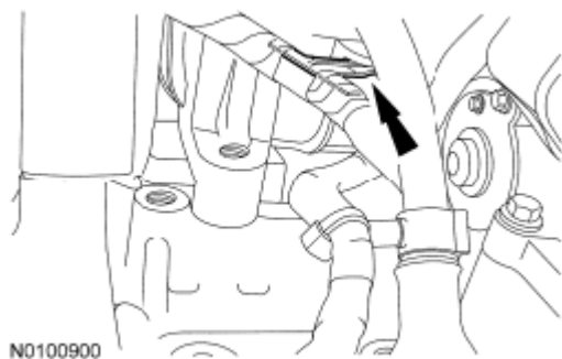
Fig. 17: Locating Engine Wiring Harness Pin-type Retainer To Intake Manifold Courtesy of FORD MOTOR CO.
