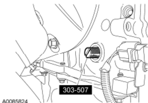
Fig. 43: Removing Crankshaft TDC Timing Peg Courtesy of FORD MOTOR CO.
