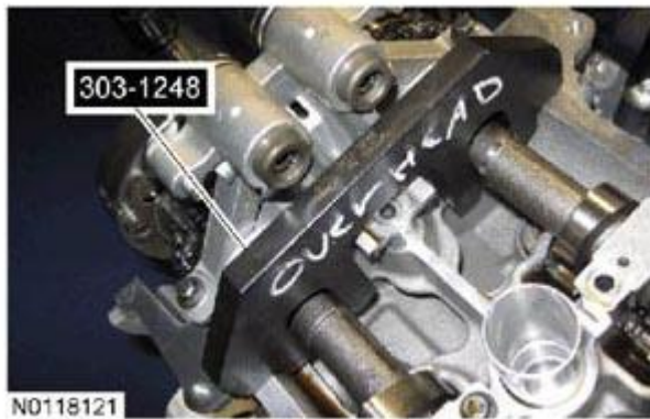
Fig. 118: Inspecting Valve Tappet Courtesy of FORD MOTOR CO.
