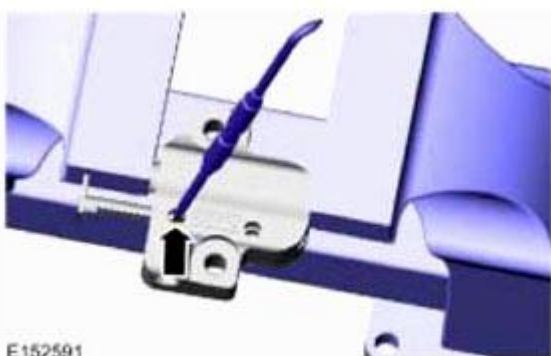
Fig. 475: Pushing Back And Hold Ratchet Mechanism Using Small Pick Courtesy of FORD MOTOR CO.
