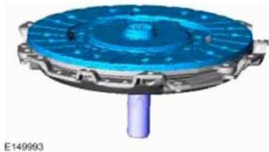
Fig. 559: Positioning Clutch Disc On Clutch Pressure Plate Courtesy of FORD MOTOR CO.
