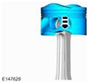
Fig. 424: Positioning Piston On Connecting Rod Courtesy of FORD MOTOR CO.
