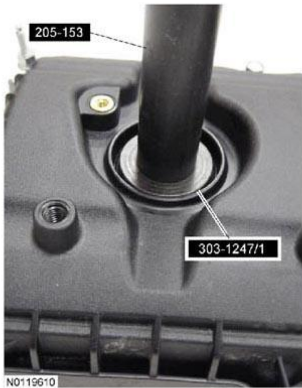
Fig. 66: Installing Camshaft Front Oil Seal Using 303-096 Installer Courtesy of FORD MOTOR CO.
