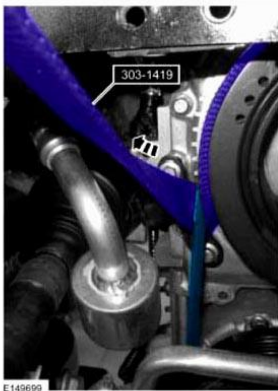
Fig. 327: Removing A/C Compressor Belt By Pulling Special Tool Courtesy of FORD MOTOR CO.
