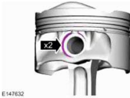
Fig. 426: Locating Piston Pin Retainers In Piston Courtesy of FORD MOTOR CO.
