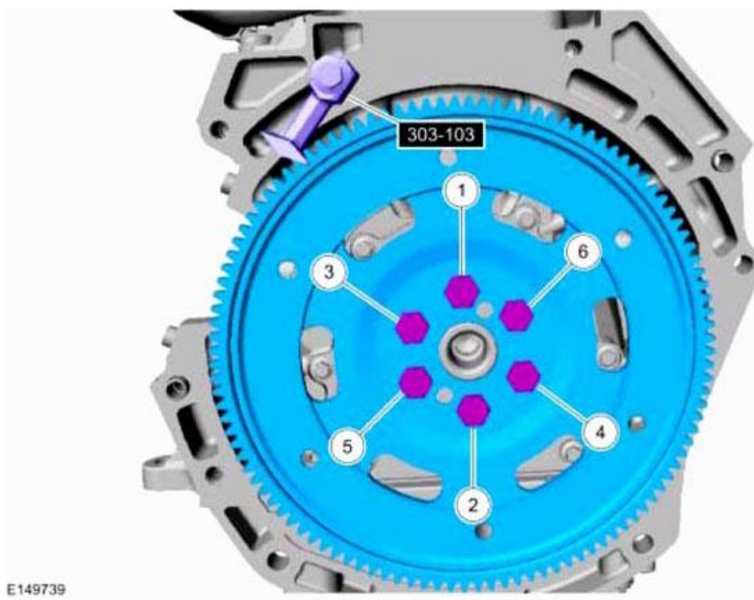
Fig. 557: Identifying 303-103 Flywheel Holding Tool And Flywheel Bolts Tightening Sequence Courtesy of FORD MOTOR CO.
