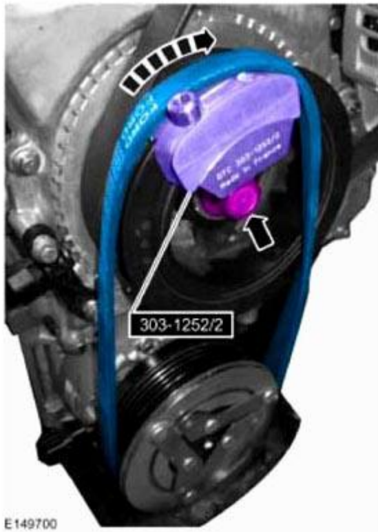
Fig. 543: Positioning A/C Compressor Belt Onto A/C Compressor Pulley And Around Special Tool On Crankshaft Pulley
