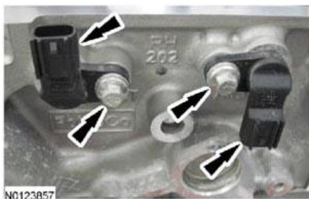
Fig. 551: Locating Engine Ground Bolt Courtesy of FORD MOTOR CO.
