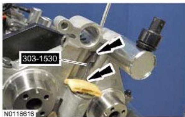
Fig. 167: Locating Engine Front Cover Bolts Courtesy of FORD MOTOR CO.
