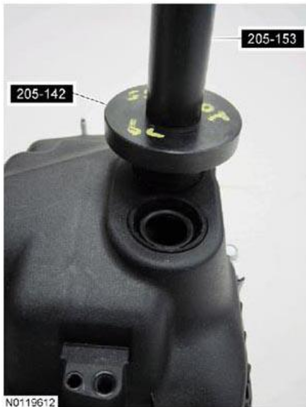
Fig. 65: Removing Crankshaft Seal From Engine Front Cover Using 303-409 Remover Courtesy of FORD MOTOR CO.
