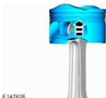
Fig. 421: Separating Piston From Connecting Rod Courtesy of FORD MOTOR CO.
