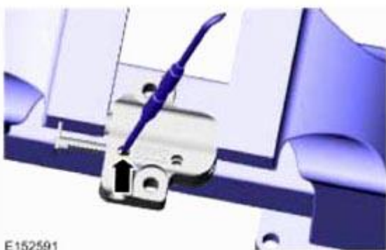
Fig. 100: Pushing Back And Hold Ratchet Mechanism Using Small Pick Courtesy of FORD MOTOR CO.
