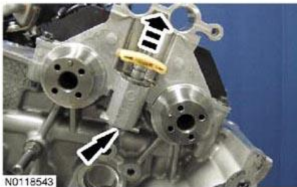
Fig. 141: Locating Engine Ground Bolt Courtesy of FORD MOTOR CO.
