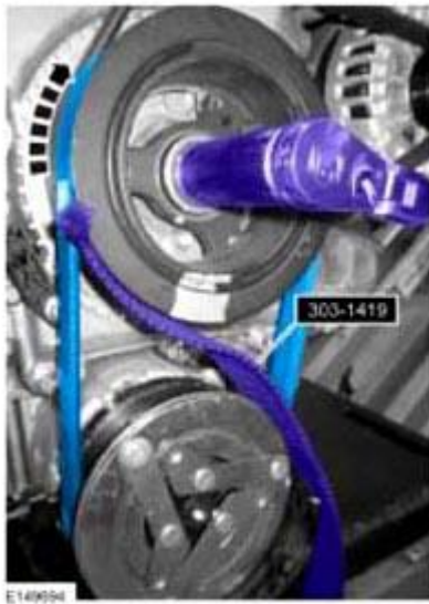
Fig. 324: Positioning Special Tool Between Crankshaft Pulley And A/C Compressor Belt Courtesy of FORD MOTOR CO.
