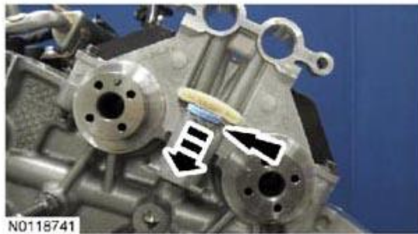
Fig. 154: Locating Transmission-To-Engine Bolts Courtesy of FORD MOTOR CO.
