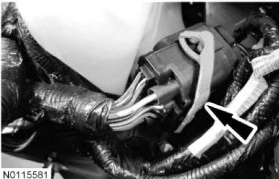
Fig. 715: Locating Engine Harness Electrical Connector Courtesy of FORD MOTOR CO.
