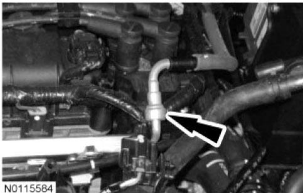
Fig. 351: Locating Fuel Tube Spring Lock Couplings From Fuel Rail Courtesy of FORD MOTOR CO.
