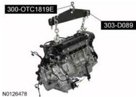
Fig. 399: Lifting Engine And Transaxle Assembly Using Floor Crane And Spreader Bar Courtesy of FORD MOTOR CO.
