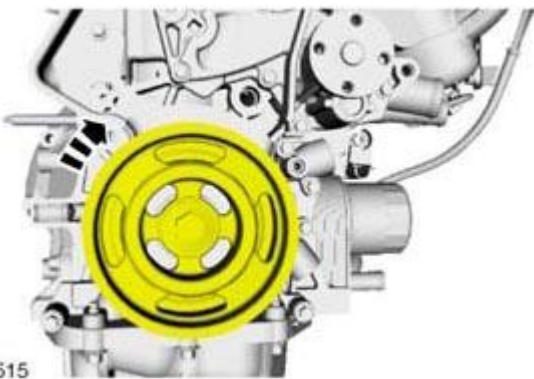
Fig. 53: Rotating Crankshaft Courtesy of FORD MOTOR CO.
