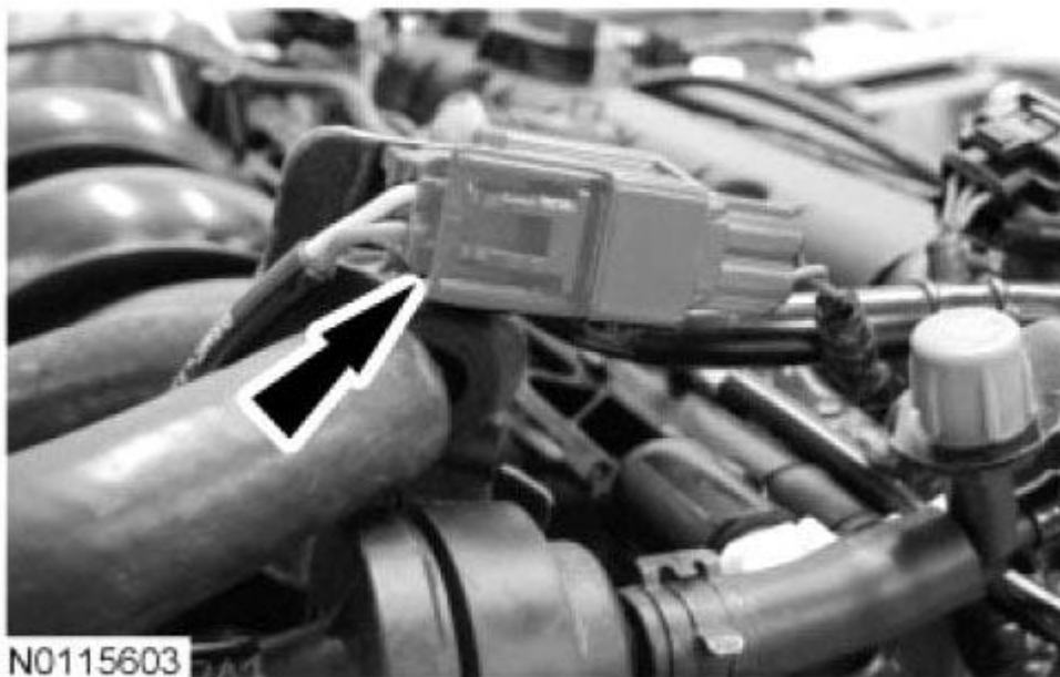
Fig. 678: Locating LH Knock Sensor (KS) Electrical Connector Courtesy of FORD MOTOR CO.
