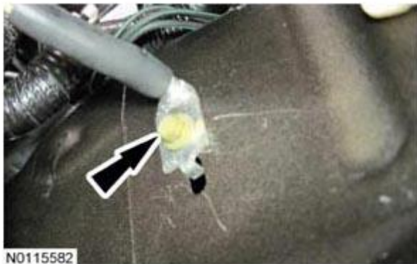
Fig. 300: Locating Bolt And Engine Ground Wire Courtesy of FORD MOTOR CO.
