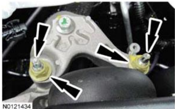
Fig. 317: Locating Engine Mount Nuts Courtesy of FORD MOTOR CO.
