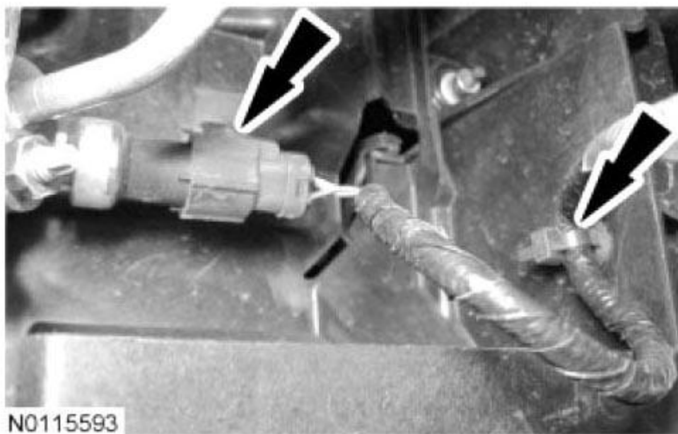
Fig. 698: Locating A/C Pressure Transducer Electrical Connector Courtesy of FORD MOTOR CO.
