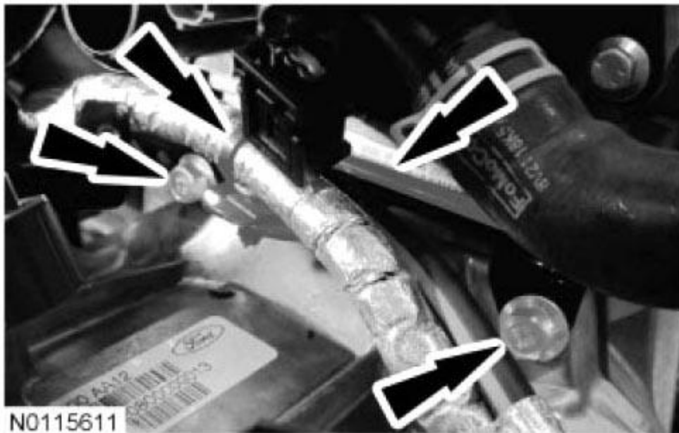
Fig. 398: Locating Upper Bellhousing-To-Engine Bolts Courtesy of FORD MOTOR CO.
