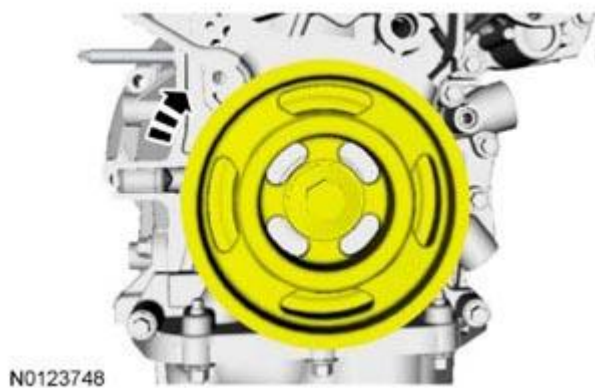
Fig. 557: Rotating Crankshaft Clockwise Courtesy of FORD MOTOR CO.
