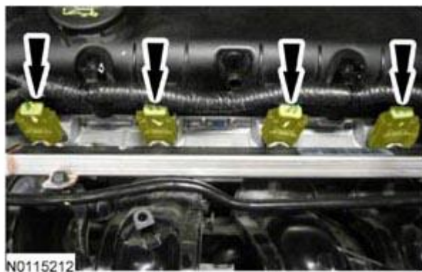
Fig. 617: Locating Fuel Injector Electrical Connectors Courtesy of FORD MOTOR CO.
