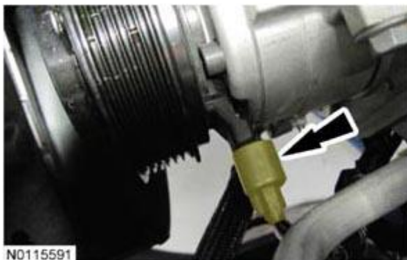
Fig. 302: Locating A/C Compressor Electrical Connector Courtesy of FORD MOTOR CO.
