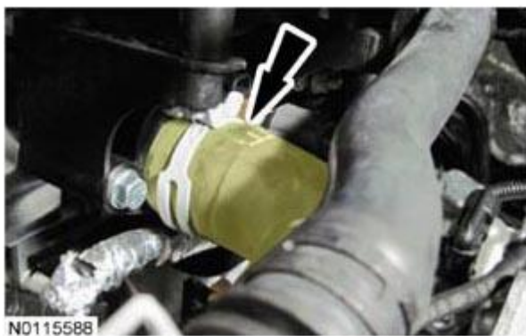
Fig. 298: Locating Upper Radiator Hose From Engine Courtesy of FORD MOTOR CO.
