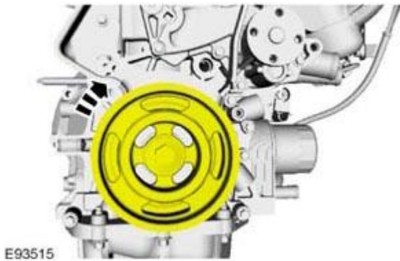
Fig. 46: Rotating Crankshaft Courtesy of FORD MOTOR CO.
