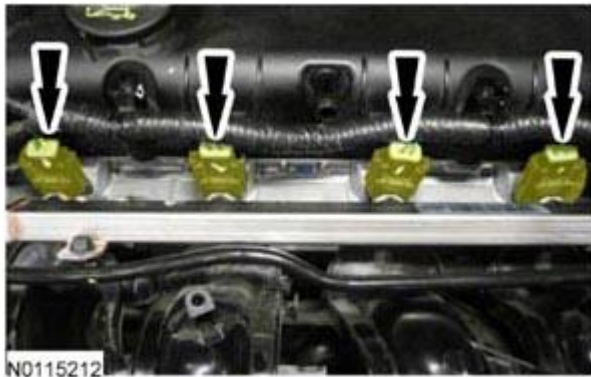
Fig. 327: Locating Fuel Injector Electrical Connectors Courtesy of FORD MOTOR CO.
