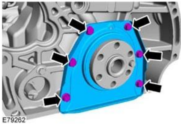
Fig. 464: Locating Bolts And Crankshaft Rear Seal Courtesy of FORD MOTOR CO.
