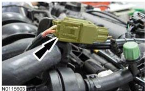
Fig. 325: Locating LH Knock Sensor (KS) Electrical Connector Courtesy of FORD MOTOR CO.
