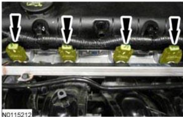
Fig. 676: Locating Fuel Injector Electrical Connectors Courtesy of FORD MOTOR CO.
