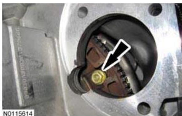
Fig. 337: Locating Flexplate-To-Clutch Nuts Courtesy of FORD MOTOR CO.
