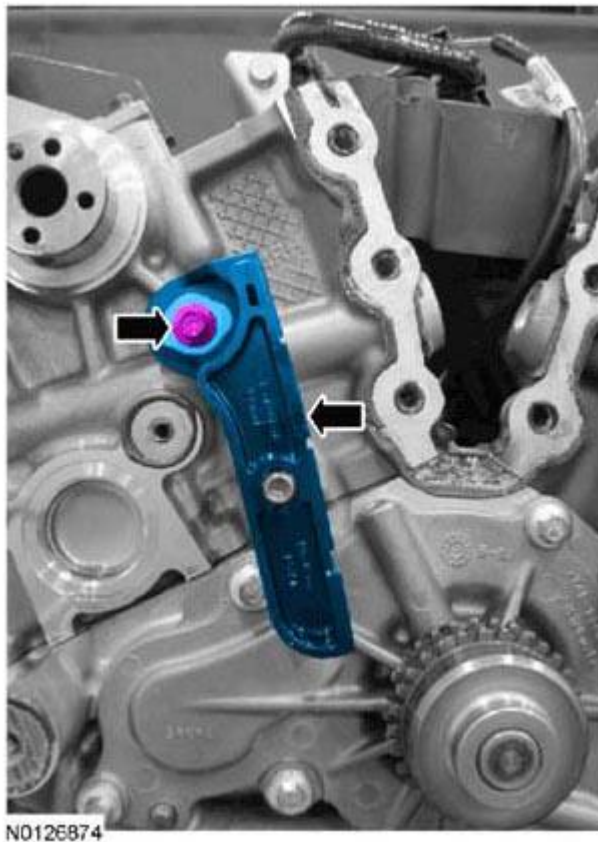
Fig. 56: Installing VCT Alignment Tool
