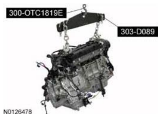
Fig. 666: Lifting Engine And Transaxle Assembly Using Floor Crane And Spreader Bar Courtesy of FORD MOTOR CO.
