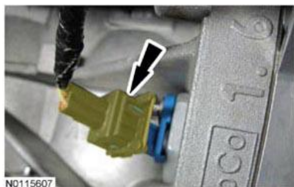
Fig. 330: Locating Crankshaft Position (CKP) Sensor Electrical Connector Courtesy of FORD MOTOR CO.
