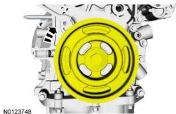
Fig. 439: Rotating Crankshaft Clockwise Courtesy of FORD MOTOR CO.
