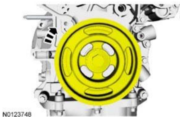
Fig. 555: Rotating Crankshaft Clockwise Courtesy of FORD MOTOR CO.
