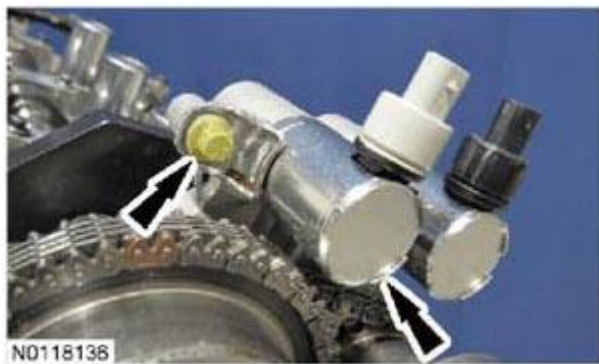
Fig. 95: Locating Bolts And Timing Belt Cover Courtesy of FORD MOTOR CO.
