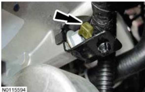
Fig. 305: Locating Wiring Harness Retainer From Lower A/C Compressor Bracket Courtesy of FORD MOTOR CO.
