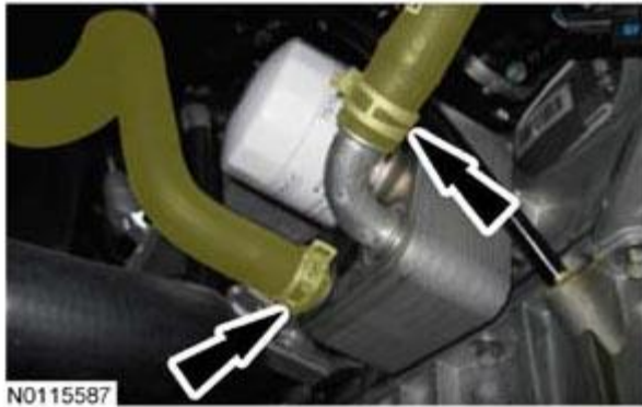
Fig. 294: Locating Coolant Hoses From Engine Oil Cooler Courtesy of FORD MOTOR CO.
