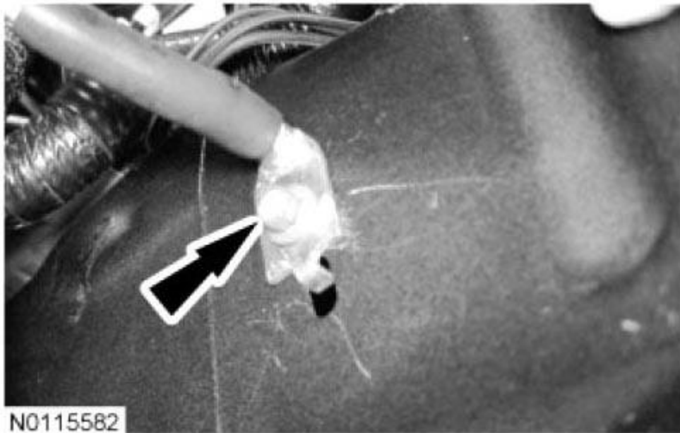
Fig. 643: Locating Bolt And Engine Ground Wire Courtesy of FORD MOTOR CO.
