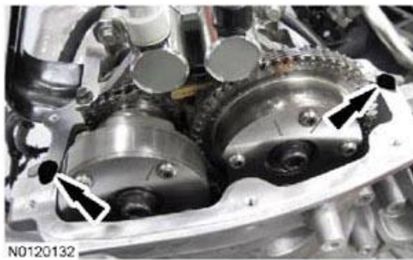
Fig. 111: Installing VCT Alignment Tool Courtesy of FORD MOTOR CO.
