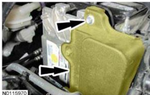
Fig. 282: Locating Bolt And PCM Cover Courtesy of FORD MOTOR CO.
