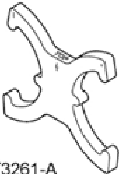
Tool, Variable Camshaft Timing (VCT) Alignment 303-1097
