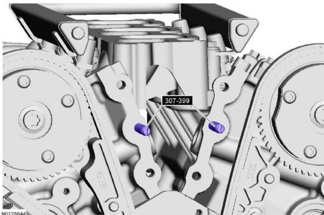
Fig. 101: Locating Bolts And Coolant Pump Pulley Courtesy of FORD MOTOR CO.
