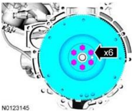
Fig. 402: Locating Bolts And Flywheel Courtesy of FORD MOTOR CO.
