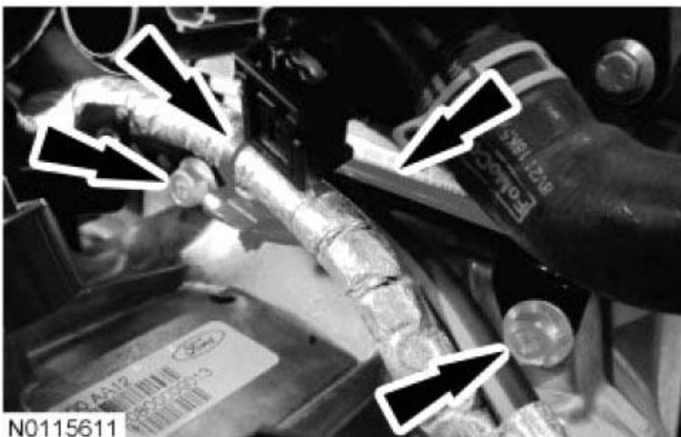
Fig. 609: Locating Upper Bellhousing-To-Engine Bolts
