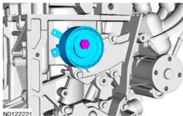
Fig. 447: Identifying Bolt And Timing Belt Tensioner Courtesy of FORD MOTOR CO.
