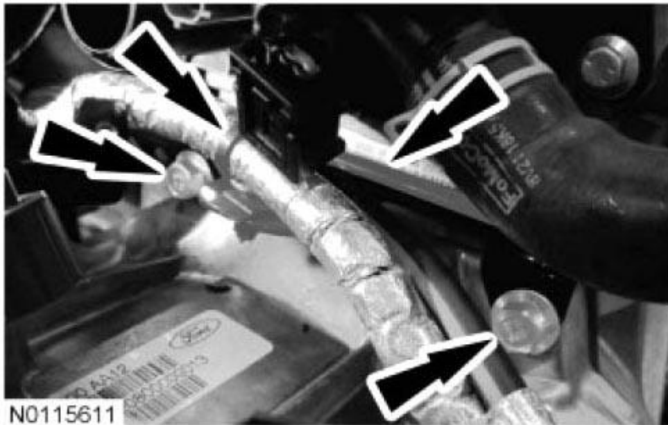
Fig. 668: Locating Upper Bellhousing-To-Engine Bolts Courtesy of FORD MOTOR CO.
