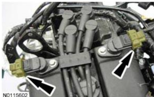
Fig. 324: Locating Camshaft Position (CMP) Sensor Electrical Connectors Courtesy of FORD MOTOR CO.
