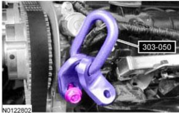
Fig. 211: Removing Engine Lifting Bracket Courtesy of FORD MOTOR CO.
