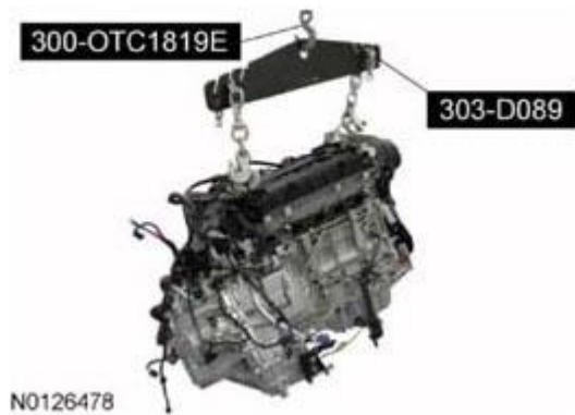
Fig. 338: Lifting Engine And Transaxle Assembly Using Floor Crane And Spreader Bar Courtesy of FORD MOTOR CO.
