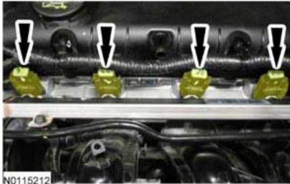
Fig. 390: Locating Fuel Injector Electrical Connectors Courtesy of FORD MOTOR CO.
