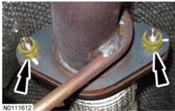
Fig. 308: Locating Catalytic Converter-To-Muffler Nuts Courtesy of FORD MOTOR CO.
