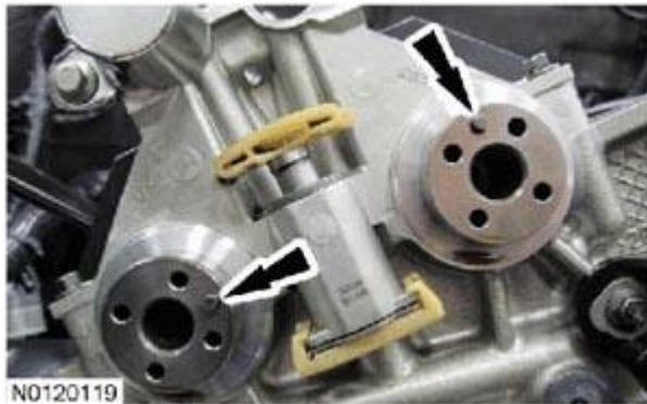
Fig. 65: Locating Bolts And Coolant Pump Pulley Courtesy of FORD MOTOR CO.
