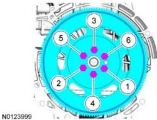
Fig. 597: Identifying Flexplate Bolts Tightening Sequence Courtesy of FORD MOTOR CO.
