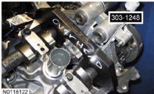
Fig. 97: Locating Bolts And Timing Belt Cover Backplate Courtesy of FORD MOTOR CO.
