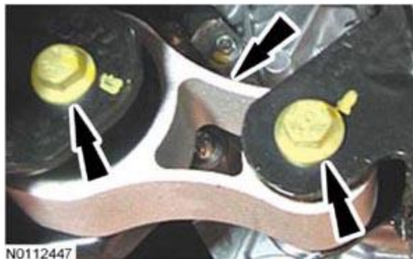
Fig. 316: Locating Bolts And Transaxle Roll Restrictor Courtesy of FORD MOTOR CO.
