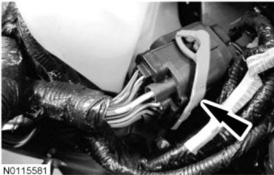
Fig. 349: Locating Engine Harness Electrical Connector Courtesy of FORD MOTOR CO.
