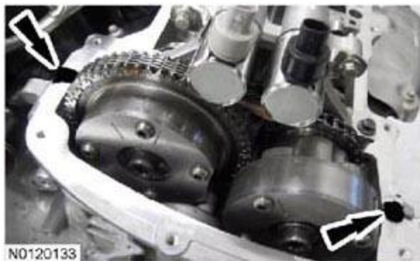
Fig. 117: Locating Bolts And Lower Timing Belt Cover Courtesy of FORD MOTOR CO.
