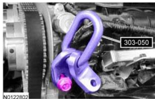
Fig. 40: Installing Engine Lifting Bracket
