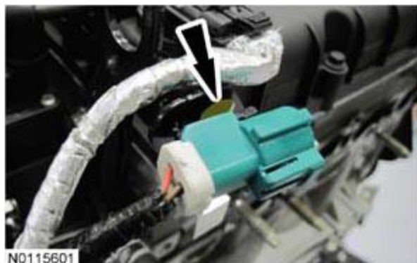
Fig. 323: Locating HO2S Sensor Electrical Connector Pin-Type Retainer From Bracket Courtesy of FORD MOTOR CO.
