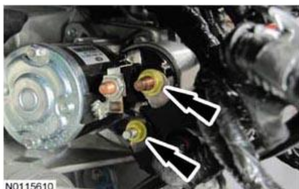
Fig. 333: Locating Nuts And Starter Motor Electrical Terminals Courtesy of FORD MOTOR CO.
