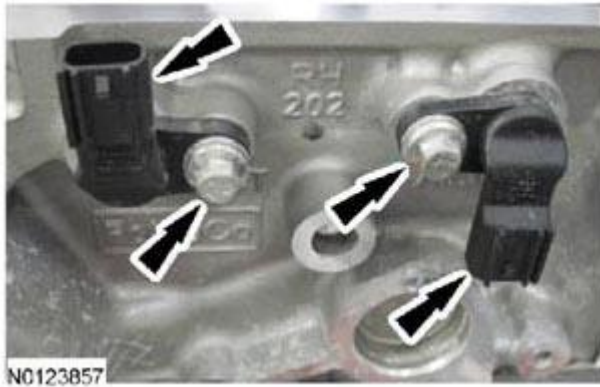
Fig. 129: Removing Camshaft Alignment Plate Courtesy of FORD MOTOR CO.
