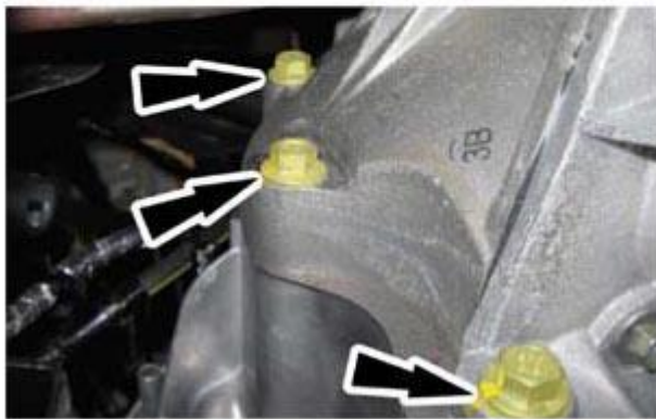
Fig. 339: Locating Clutch Housing-To-Engine Bolts Courtesy of FORD MOTOR CO.
