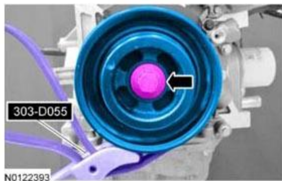
Fig. 554: Locating Crankshaft Bolt Courtesy of FORD MOTOR CO.
