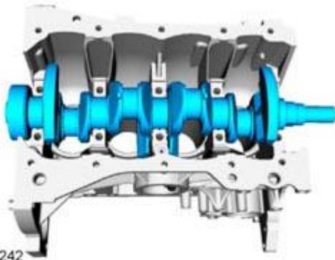
Fig. 472: Identifying Crankshaft And Engine Block Courtesy of FORD MOTOR CO.
