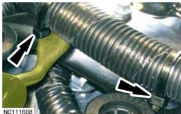
Fig. 285: Locating Positive Battery Cable Wire Harness Retainers From Battery Tray Bracket Courtesy of FORD MOTOR CO.
