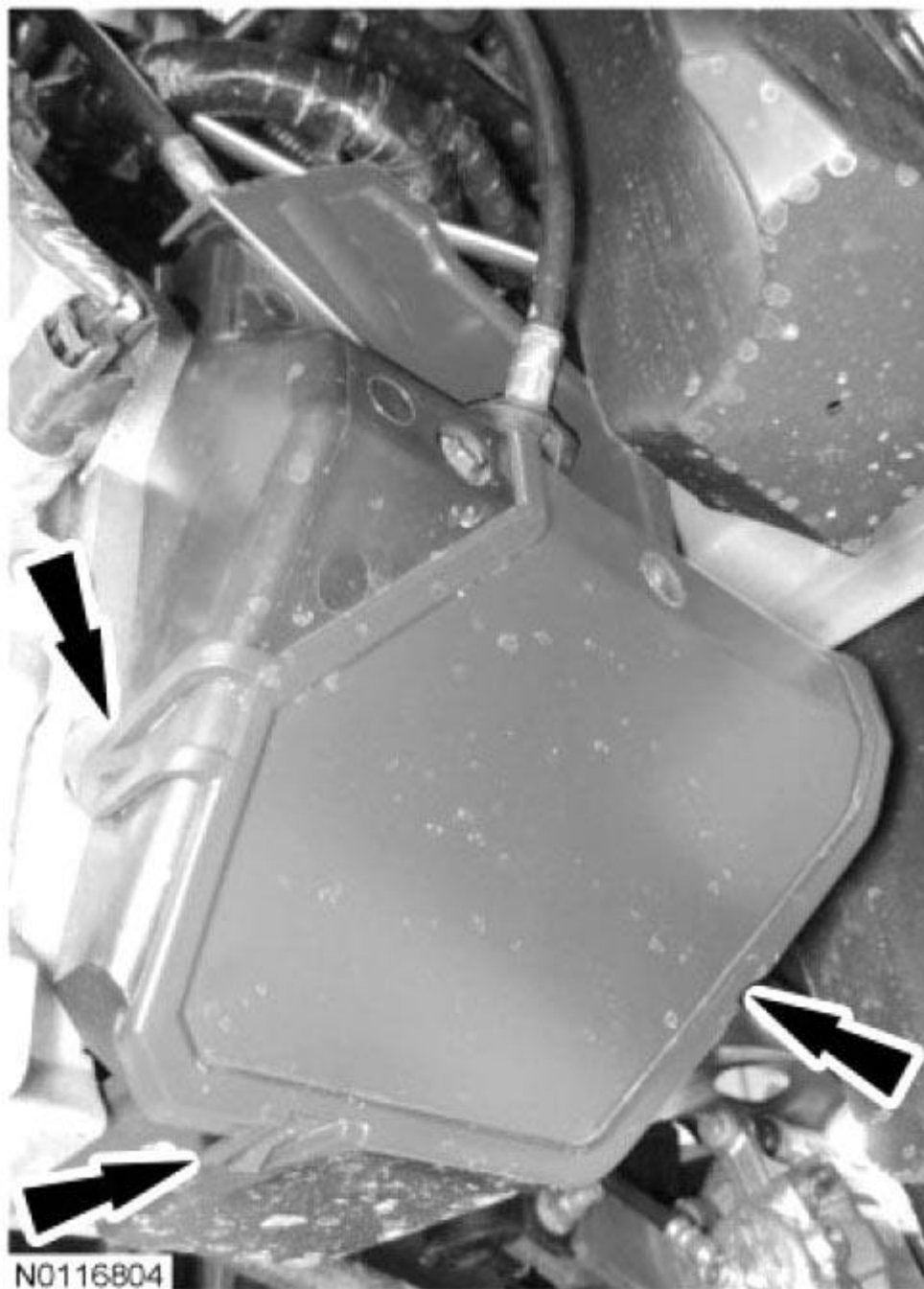
Fig. 725: Locating Retainers And Gearshift Cable Cover Courtesy of FORD MOTOR CO.
