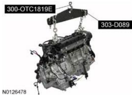
Fig. 605: Lifting Engine And Transaxle Assembly Using Floor Crane And Spreader Bar Courtesy of FORD MOTOR CO.
