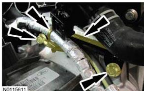
Fig. 335: Locating Upper Bellhousing-To-Engine Bolts Courtesy of FORD MOTOR CO.
