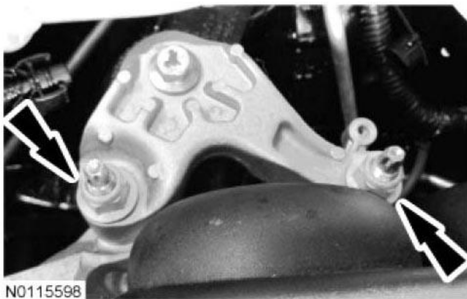
Fig. 686: Locating Engine Mount And Nuts Courtesy of FORD MOTOR CO.
