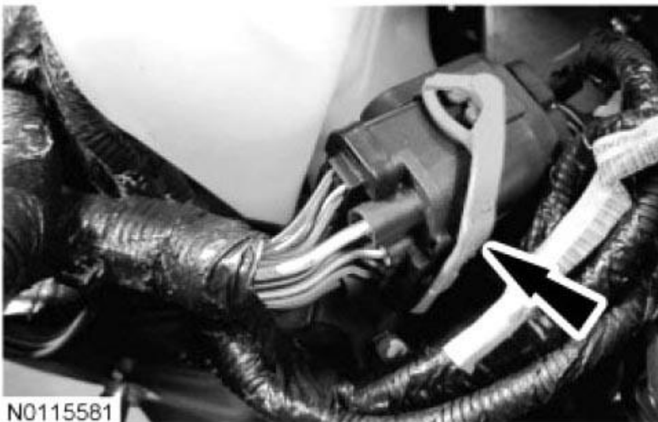
Fig. 656: Locating Engine Harness Electrical Connector Courtesy of FORD MOTOR CO.
