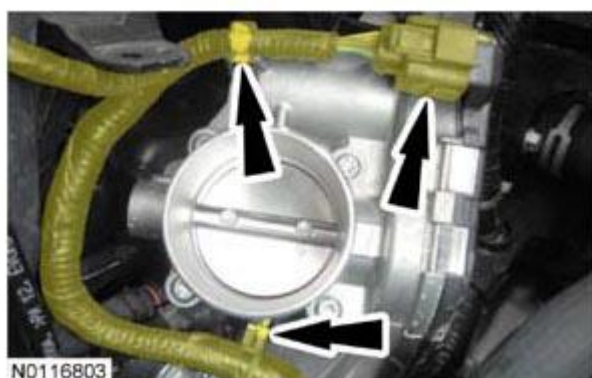
Fig. 329: Locating Throttle Body (TB) Electrical Connector Courtesy of FORD MOTOR CO.
