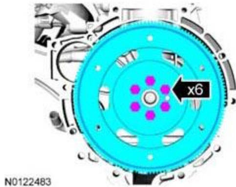
Fig. 403: Locating Bolts And Flexplate Courtesy of FORD MOTOR CO.
