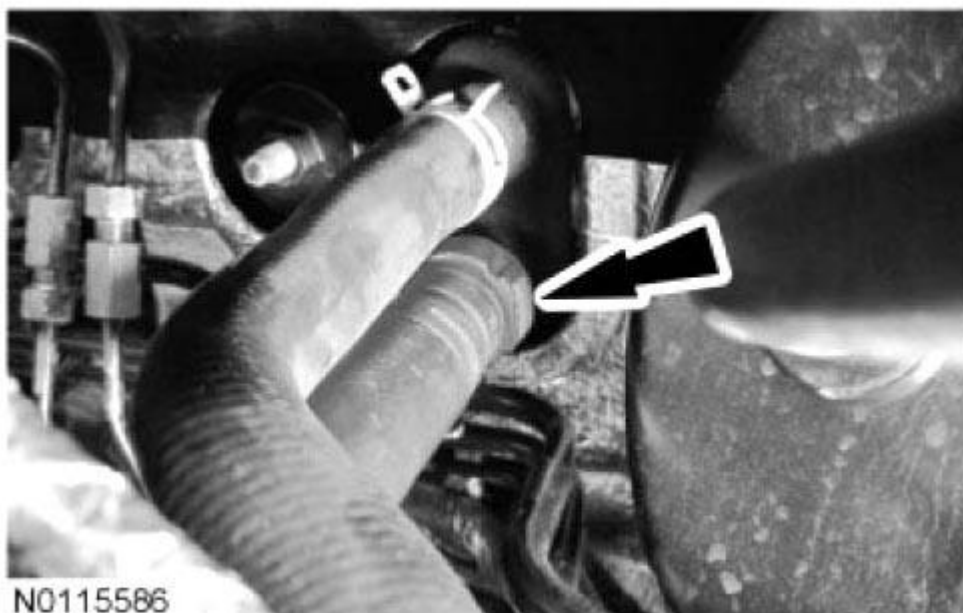
Fig. 648: Locating Lower Heater Hose To Heater Core Courtesy of FORD MOTOR CO.
