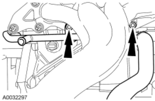
Fig. 320: Locating Coolant Tube Nuts Courtesy of FORD MOTOR CO.
