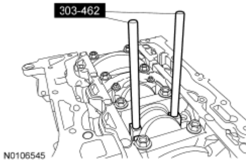
Fig. 212: Removing Piston/Rod Assembly From Engine Block Courtesy of FORD MOTOR CO.
