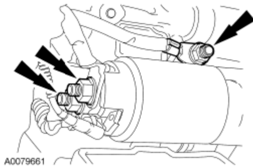
Fig. 359: Locating Positive And Negative Battery Cable Courtesy of FORD MOTOR CO.
