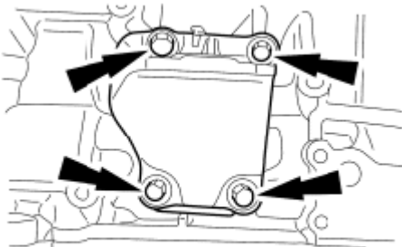
Fig. 183: Locating LH Engine Mount Bracket Bolts Courtesy of FORD MOTOR CO.
