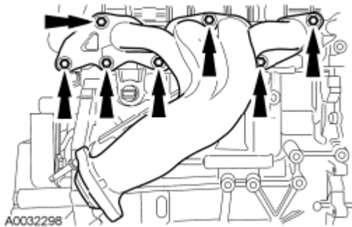
Fig. 319: Locating Exhaust Manifold Nuts Courtesy of FORD MOTOR CO.
