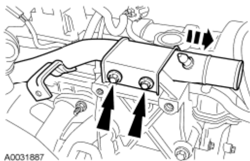
Fig. 82: Removing Front Coolant Outlet Pipe Courtesy of FORD MOTOR CO.
