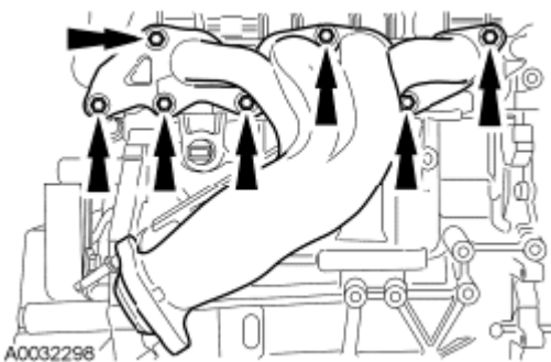
Fig. 165: Locating Exhaust Manifold Nuts Courtesy of FORD MOTOR CO.
