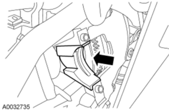
Fig. 338: Locating Starter Dust Shield Courtesy of FORD MOTOR CO.
