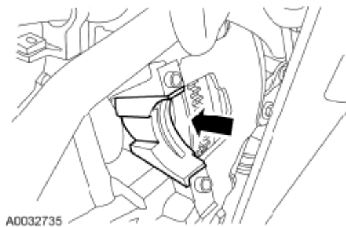
Fig. 337: Locating Starter Dust Shield Courtesy of FORD MOTOR CO.
