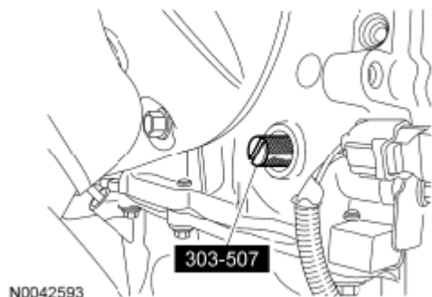
Fig. 291: Removing Crankshaft Timing Peg Courtesy of FORD MOTOR CO.
