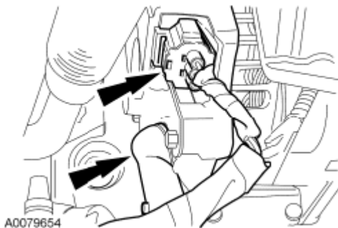
Fig. 127: Locating Generator Electrical Connections Courtesy of FORD MOTOR CO.
