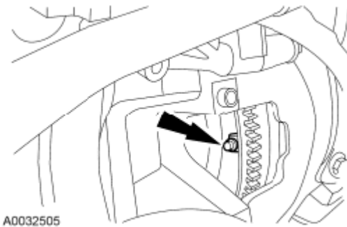
Fig. 333: Locating Torque Converter Nuts Courtesy of FORD MOTOR CO.
