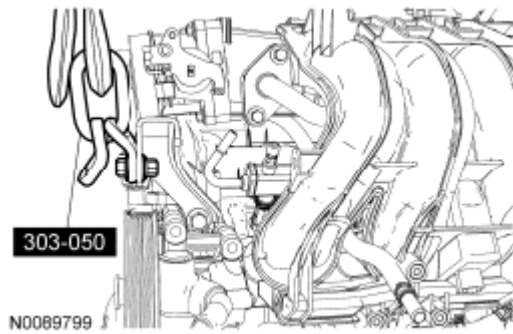
Fig. 151: Identifying Engine Lifting Brackets Courtesy of FORD MOTOR CO.
