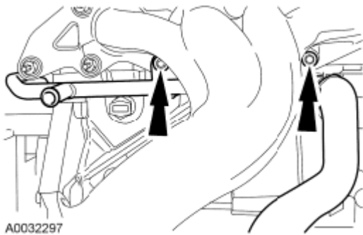
Fig. 163: Locating Coolant Tube Assembly Nuts Courtesy of FORD MOTOR CO.
