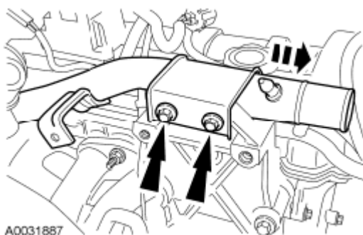
Fig. 81: Locating Front Coolant Outlet Pipe Bolts Courtesy of FORD MOTOR CO.
