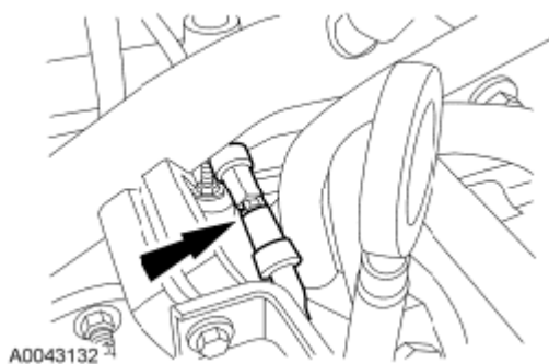
Fig. 368: Locating Vacuum Reservoir Tube Courtesy of FORD MOTOR CO.
