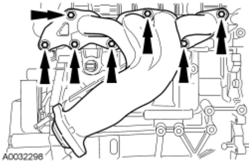
Fig. 318: Locating Exhaust Manifold Nuts Courtesy of FORD MOTOR CO.
