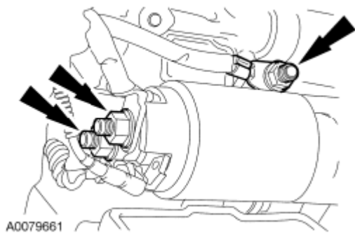
Fig. 124: Locating Starter Cable Nuts Courtesy of FORD MOTOR CO.
