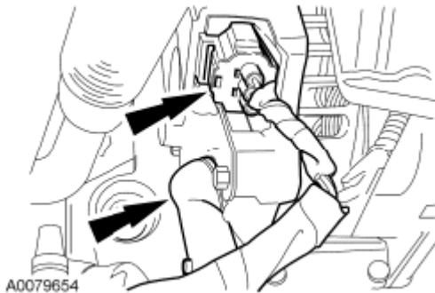
Fig. 355: Locating Generator Electrical Connections Courtesy of FORD MOTOR CO.
