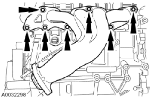
Fig. 164: Locating Exhaust Manifold Nuts Courtesy of FORD MOTOR CO.
