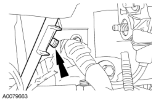
Fig. 318: Locating Generator Wiring Pin-Type Retainer Courtesy of FORD MOTOR CO.
