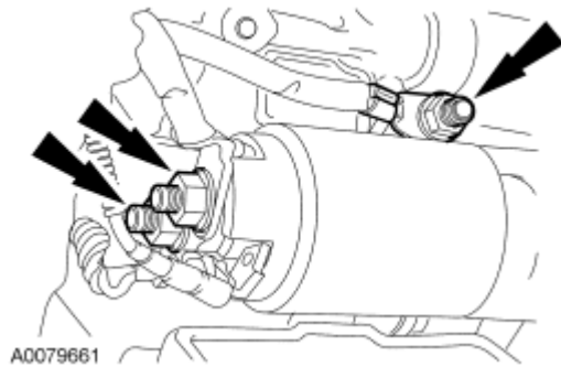
Fig. 118: Locating Solenoid Control Wire & Nut Courtesy of FORD MOTOR CO.
