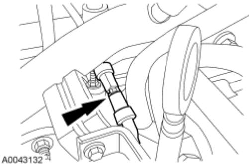
Fig. 108: Locating Vacuum Reservoir Tube Connection Courtesy of FORD MOTOR CO.
