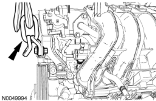
Fig. 145: Locating Engine Lifting Bracket Courtesy of FORD MOTOR CO.
