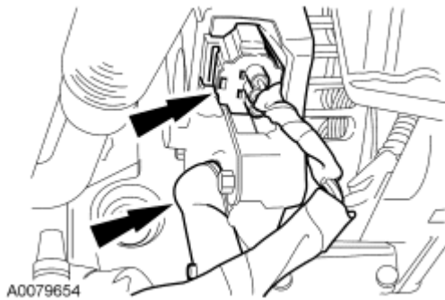
Fig. 319: Locating Generator Electrical Connections Courtesy of FORD MOTOR CO.
