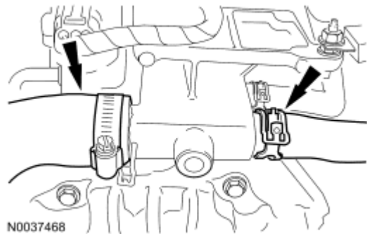
Fig. 609: Locating Upper Radiator And Heater Hoses Courtesy of FORD MOTOR CO.
