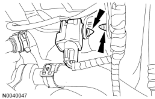
Fig. 566: Locating Knock Sensor (KS) Electrical Connector And Harness Pin-Type Retainers Courtesy of FORD MOTOR CO.
