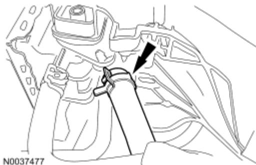
Fig. 237: Locating Power Steering Cooler Tube Courtesy of FORD MOTOR CO.
