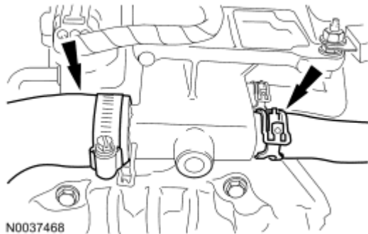
Fig. 667: Locating Upper Radiator And Heater Hoses Courtesy of FORD MOTOR CO.
