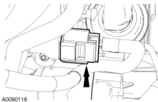
Fig. 363: Locating Manifold Actual Pressure (MAP) Sensor Electrical Connector Courtesy of FORD MOTOR CO.
