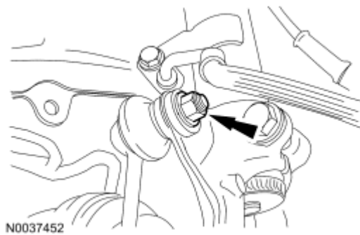
Fig. 212: Locating Sway Bar Links And Nuts Courtesy of FORD MOTOR CO.
