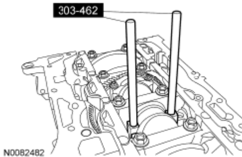
Fig. 419: Identifying Connecting Rod Installer
