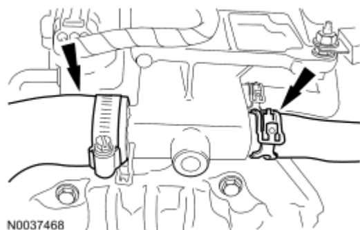
Fig. 294: Locating Upper Radiator And Heater Hoses Courtesy of FORD MOTOR CO.
