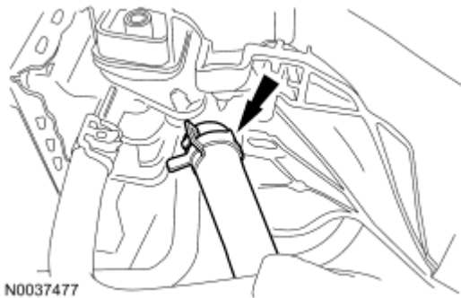
Fig. 300: Locating Power Steering Cooler Tube Courtesy of FORD MOTOR CO.
