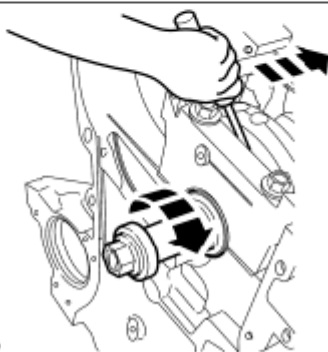
Fig. 14: Measuring Gear Backlash
