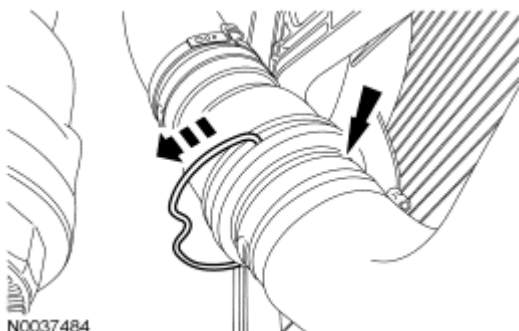
Fig. 307: Removing Retaining Clip And Locating Lower Radiator Hose Courtesy of FORD MOTOR CO.
