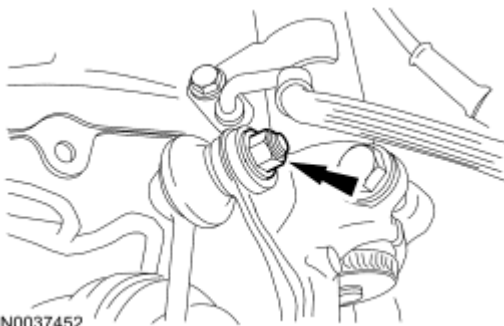
Fig. 626: Locating Sway Bar Links And Nuts
