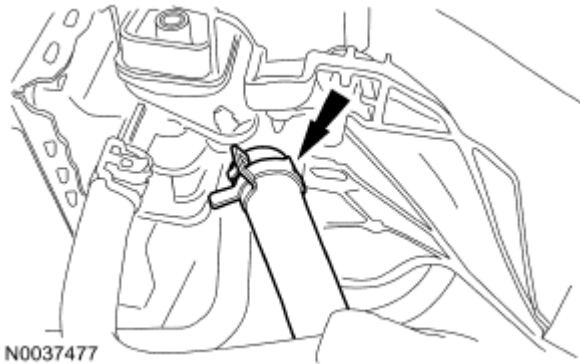
Fig. 298: Locating Power Steering Cooler Tube Courtesy of FORD MOTOR CO.
