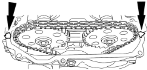
Fig. 464: Locating Silicone Gasket Applying Area Courtesy of FORD MOTOR CO.
