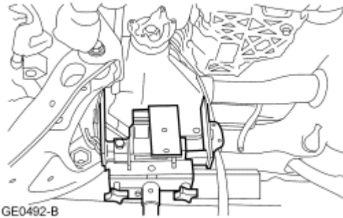
Fig. 93: Securing Front Axle Housing To Suitable Jack Courtesy of FORD MOTOR CO.
