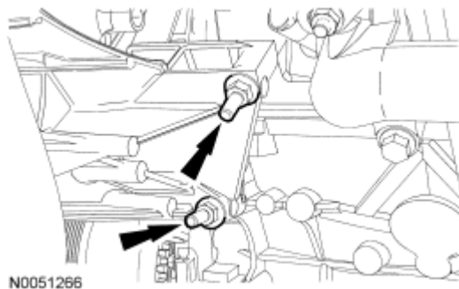
Fig. 348: Locating Stud Bolts Courtesy of FORD MOTOR CO.
