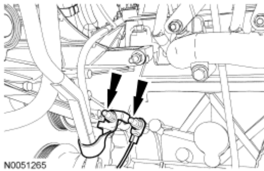
Fig. 135: Locating Ground Wire & Wiring Harness Bracket Courtesy of FORD MOTOR CO.
