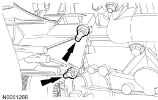
Fig. 136: Locating Stud Bolts Courtesy of FORD MOTOR CO.
