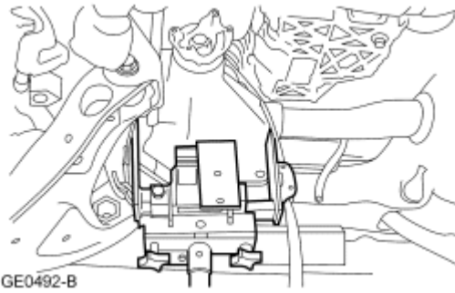
Fig. 112: Securing Front Axle Housing To Suitable Jack Courtesy of FORD MOTOR CO.
