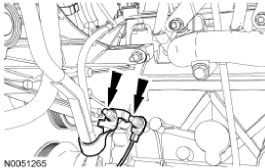
Fig. 349: Locating Wiring Harness Bracket, Ground Strap & Nuts Courtesy of FORD MOTOR CO.
