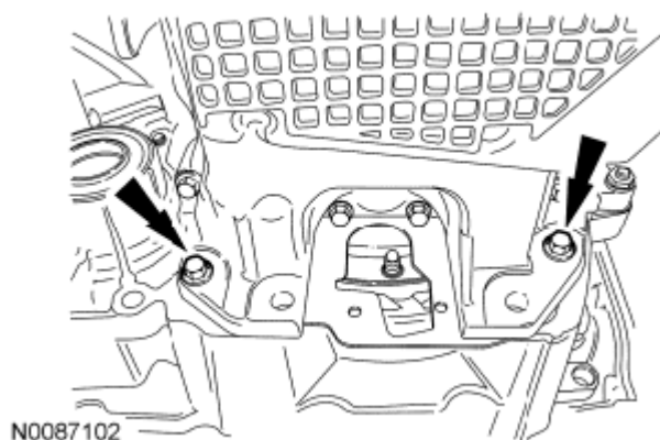
Fig. 423: Locating Oil Pan-To-Transaxle Bolts Courtesy of FORD MOTOR CO.
