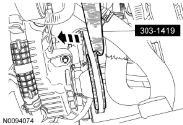
Fig. 223: Pulling Stretchy Belt Remover Courtesy of FORD MOTOR CO.
