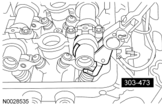
Fig. 92: Identifying Valve Spring Compressor Courtesy of FORD MOTOR CO.
