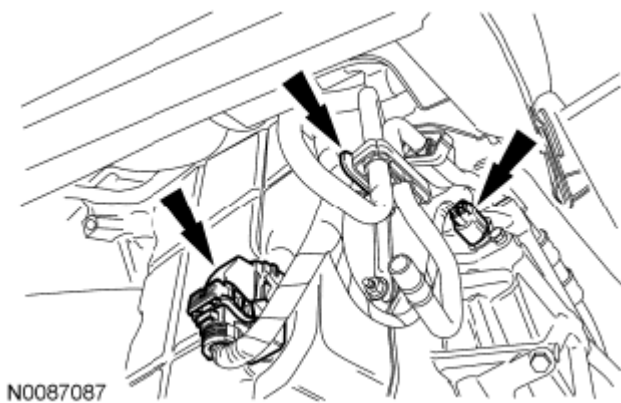
Fig. 441: Locating Transmission Electrical Connectors And Wiring Retainer Courtesy of FORD MOTOR CO.
