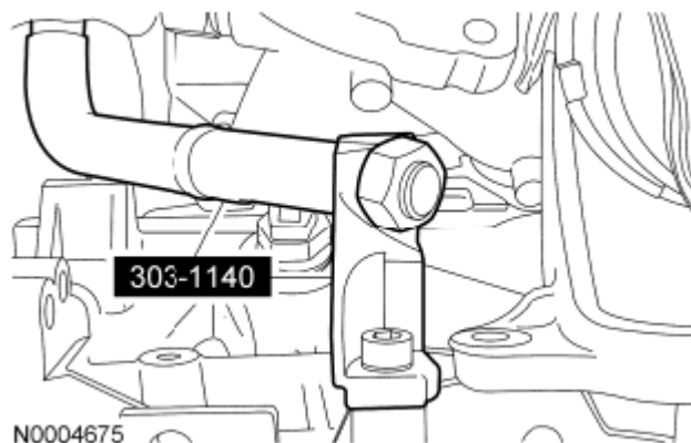
Fig. 175: Identifying Upper Half Of Engine Lifting Bracket Set Courtesy of FORD MOTOR CO.
