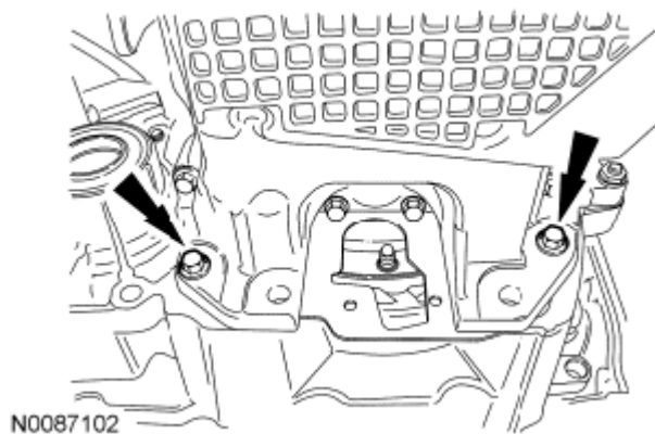
Fig. 154: Locating Oil Pan-To-Transaxle Bolts Courtesy of FORD MOTOR CO.
