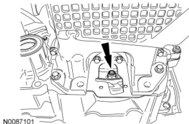
Fig. 153: Locating Torque Converter Nuts Courtesy of FORD MOTOR CO.
