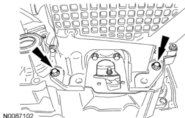
Fig. 153: Locating Oil Pan-To-Transaxle Bolts Courtesy of FORD MOTOR CO.
