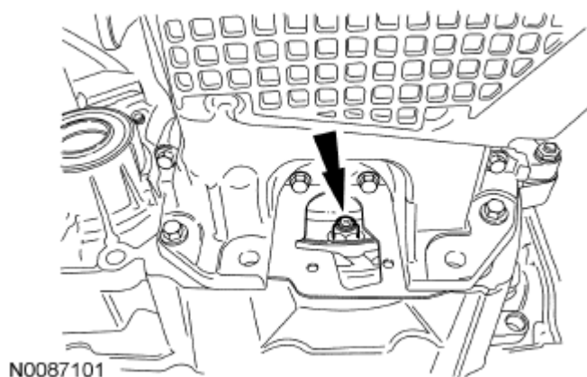
Fig. 424: Locating Torque Converter Nuts Courtesy of FORD MOTOR CO.
