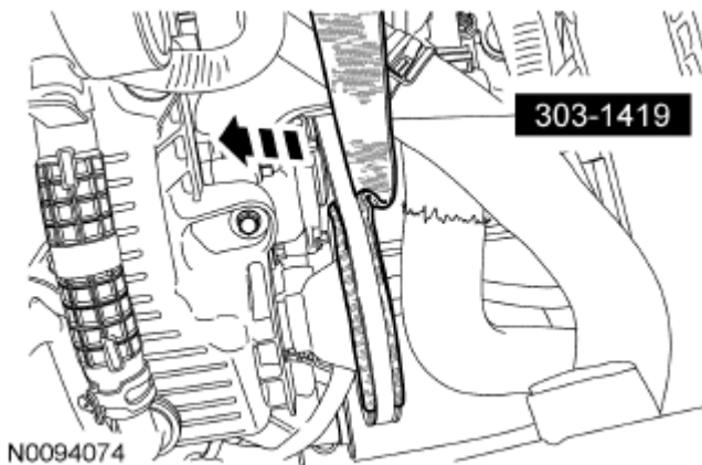
Fig. 222: Removing Coolant Pump Belt Courtesy of FORD MOTOR CO.
