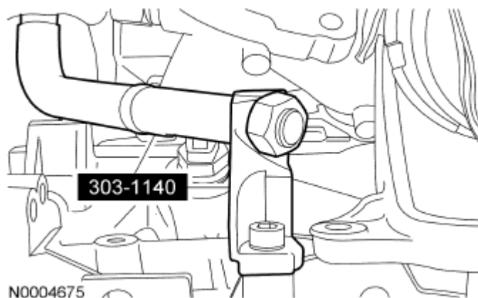
Fig. 174: Identifying Upper Half Of Lifting Hook Courtesy of FORD MOTOR CO.
