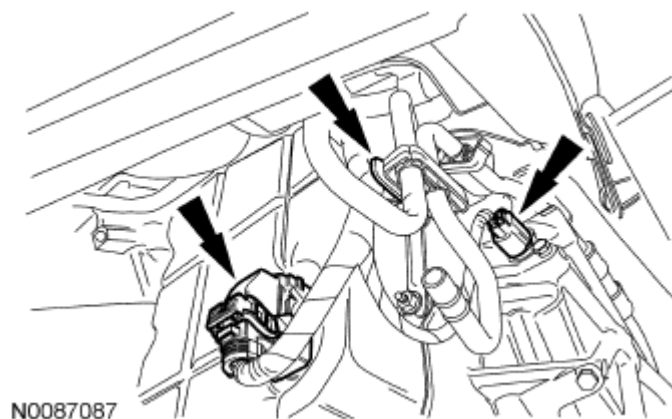
Fig. 136: Locating Transmission Electrical Connector Courtesy of FORD MOTOR CO.
