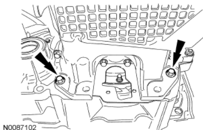
Fig. 422: Locating Oil Pan-To-Transaxle Bolts Courtesy of FORD MOTOR CO.
