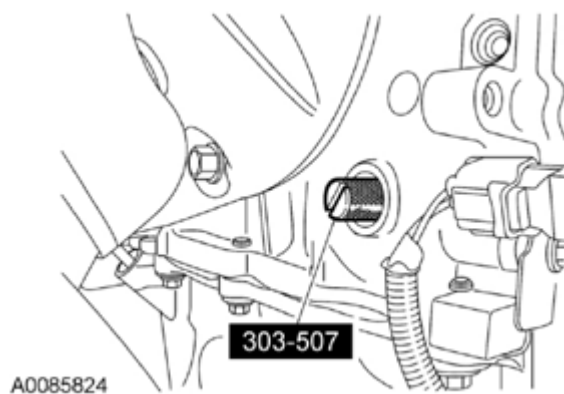
Fig. 477: Identifying Crankshaft TDC Timing Peg Courtesy of FORD MOTOR CO.
