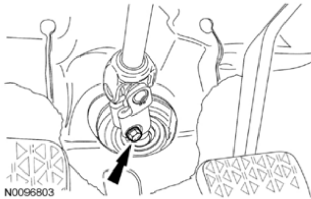
Fig. 260: Locating Steering Column Shaft Bolt Courtesy of FORD MOTOR CO.
