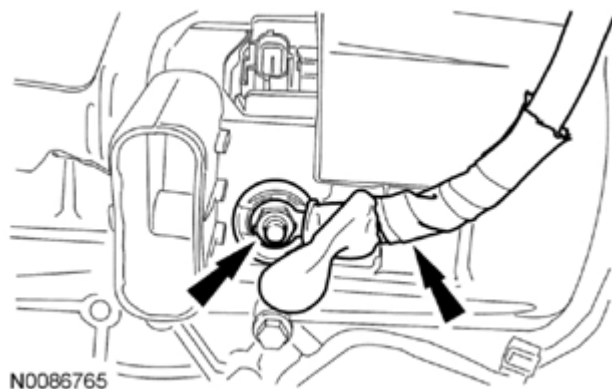
Fig. 544: Locating Nut And Generator B+ Wiring Harness Courtesy of FORD MOTOR CO.
