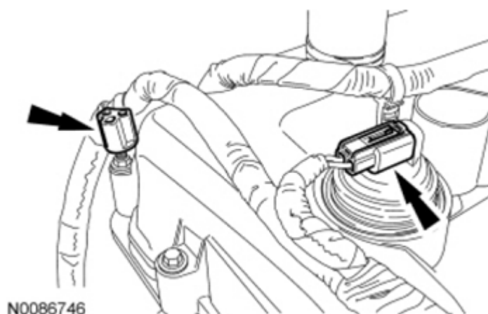
Fig. 255: Locating VCT Oil Control Solenoid Electrical Connector And Wiring Harness Retainer Courtesy of FORD MOTOR CO.
