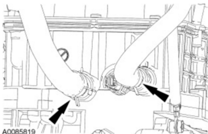
Fig. 498: Locating Transaxle Coolant Hoses Courtesy of FORD MOTOR CO.
