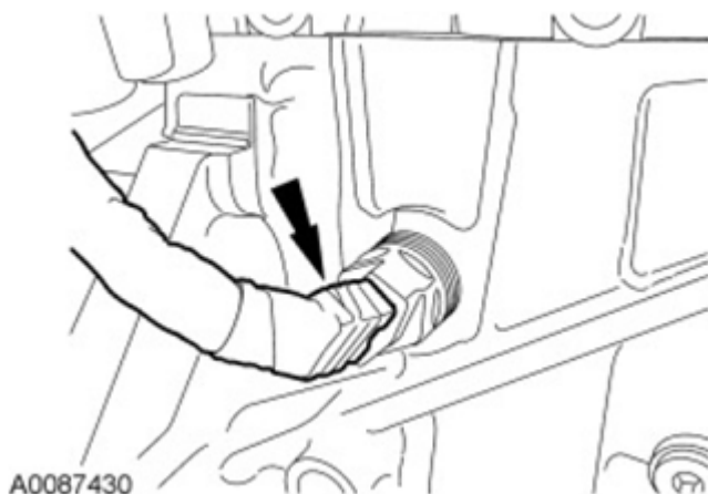
Fig. 509: Locating Block Heater Electrical Connector Courtesy of FORD MOTOR CO.
