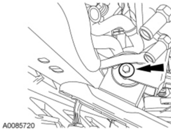
Fig. 485: Locating Lower Transaxle Insulator Through Bolt Courtesy of FORD MOTOR CO.
