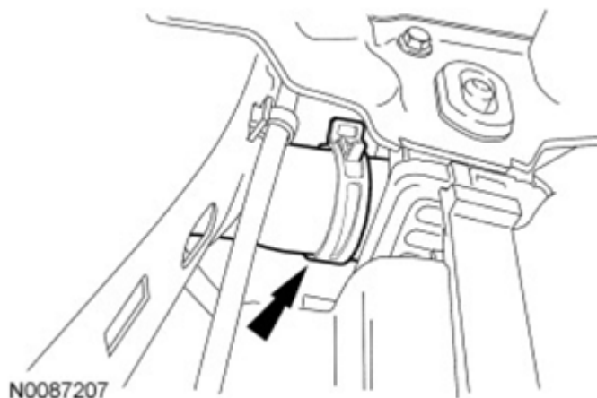
Fig. 192: Locating Upper Radiator Coolant Hose Courtesy of FORD MOTOR CO.
