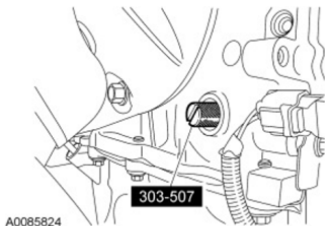
Fig. 40: Locating Crankshaft TDC Timing Peg Courtesy of FORD MOTOR CO.
