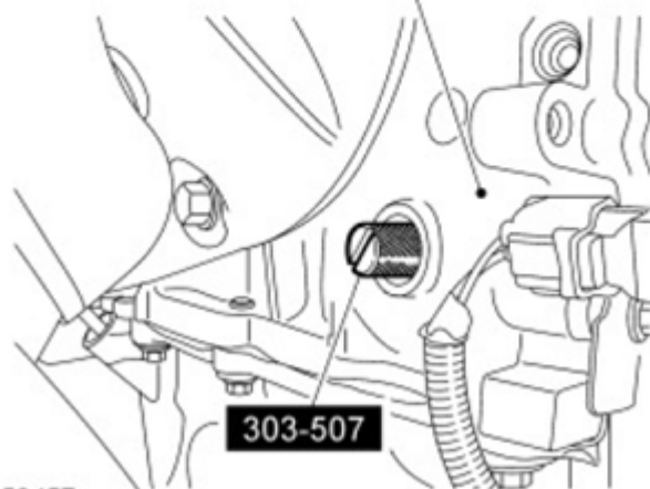
Fig. 316: Remove/Install Crankshaft TDC Timing Peg Courtesy of FORD MOTOR CO.
