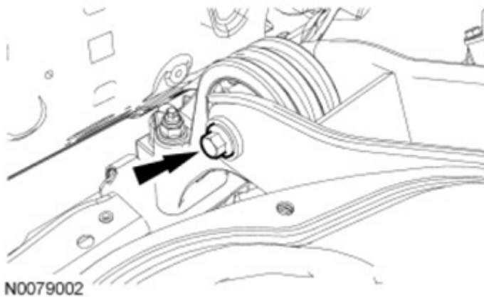
Fig. 480: Locating Rear Transaxle Insulator Through Bolt Courtesy of FORD MOTOR CO.
