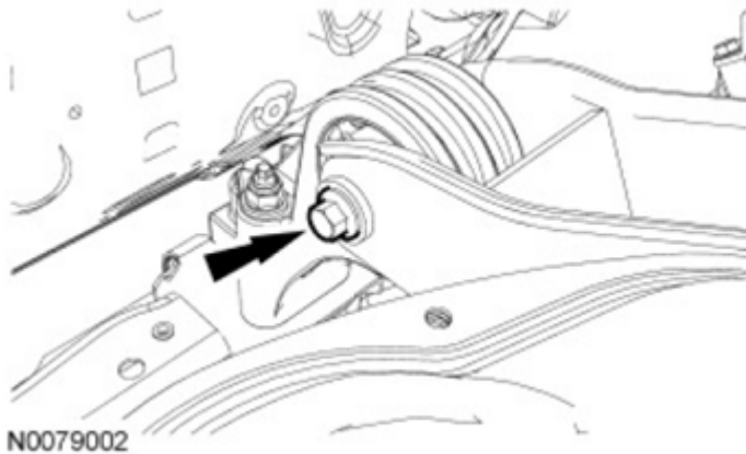
Fig. 223: Locating Rear Transaxle Insulator Through Bolt Courtesy of FORD MOTOR CO.
