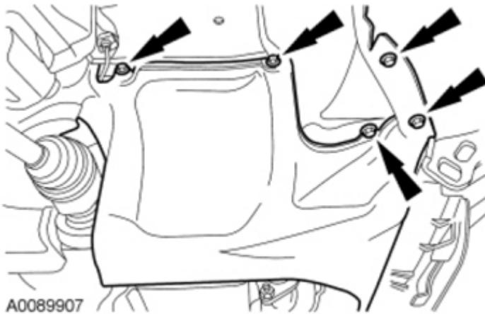
Fig. 160: Locating RH Splash Shield And Retainers Courtesy of FORD MOTOR CO.
