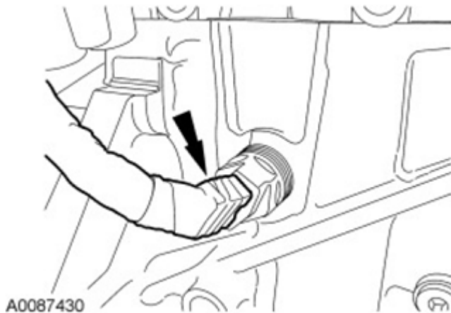
Fig. 195: Locating Block Heater Electrical Connector Courtesy of FORD MOTOR CO.
