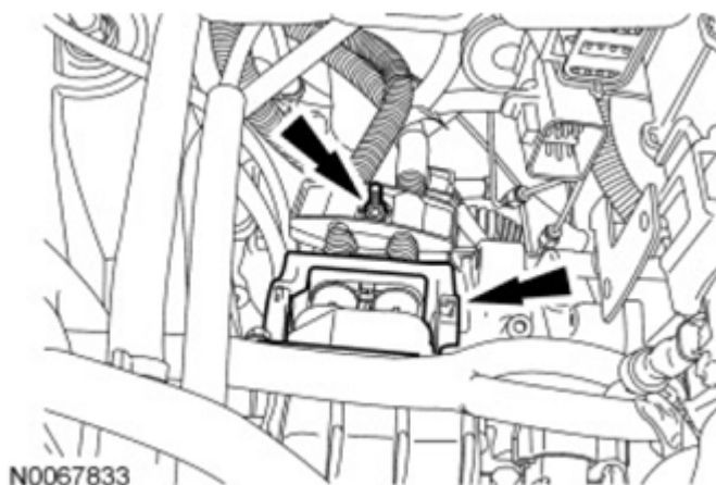
Fig. 506: Locating Stud Bolt And Transaxle Harness Electrical Connector Courtesy of FORD MOTOR CO.
