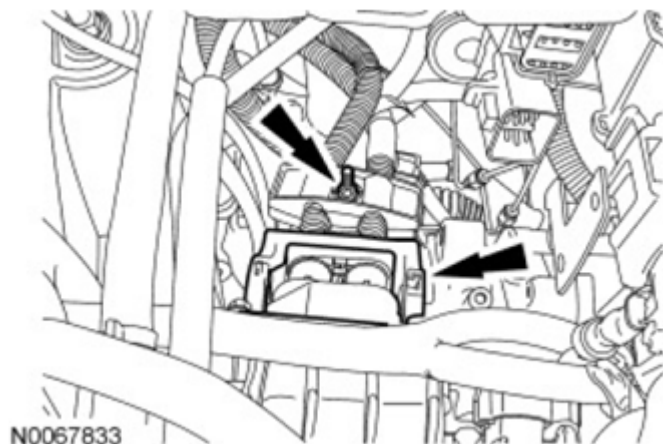
Fig. 198: Locating Stud Bolt And Transaxle Harness Electrical Connector Courtesy of FORD MOTOR CO.
