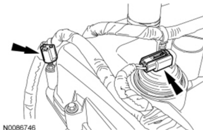
Fig. 447: Locating VCT Oil Control Solenoid Electrical Connector And Wiring Harness Retainer Courtesy of FORD MOTOR CO.
