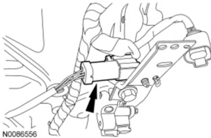
Fig. 238: Locating Catalyst Monitor Sensor Electrical Connector Courtesy of FORD MOTOR CO.
