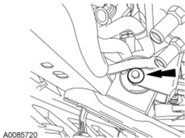
Fig. 218: Locating Lower Transaxle Insulator Through Bolt Courtesy of FORD MOTOR CO.
