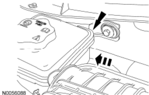
Fig. 735: Attaching Power Steering Reservoir Onto Cowl Courtesy of FORD MOTOR CO.
