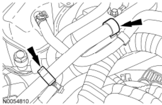
Fig. 745: Locating Coolant Tube Retainer Clips & A/C Tube Courtesy of FORD MOTOR CO.
