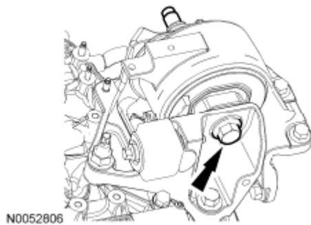
Fig. 698: Locating Transaxle Support Insulator Through Bolt & Nut Courtesy of FORD MOTOR CO.
