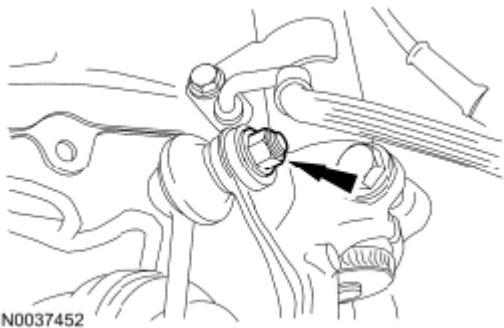
Fig. 100: Locating Stabilizer Bar Links & Nuts
