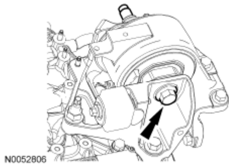
Fig. 175: Locating Transaxle Support Insulator Through Bolt & Nut Courtesy of FORD MOTOR CO.
