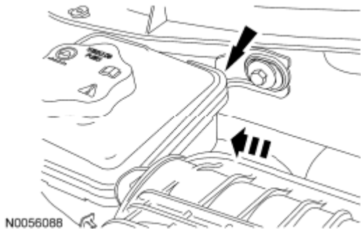
Fig. 822: Attaching Power Steering Reservoir Onto Cowl Courtesy of FORD MOTOR CO.
