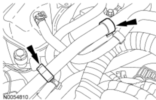
Fig. 832: Locating Coolant Tube Retainer Clips & A/C Tube Courtesy of FORD MOTOR CO.
