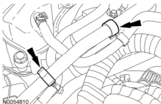
Fig. 136: Locating Coolant Tube Retainer Clips & A/C Tube Courtesy of FORD MOTOR CO.
