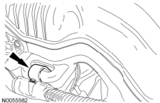
Fig. 791: Locating Block Heater Wiring Harness Retainer To Upper Intake Manifold Courtesy of FORD MOTOR CO.
