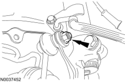
Fig. 803: Locating Stabilizer Bar Links & Nuts Courtesy of FORD MOTOR CO.
