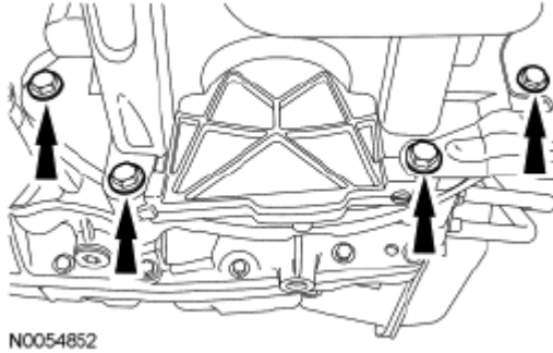
Fig. 93: Locating Oil Pan-To-Transaxle Bolts Courtesy of FORD MOTOR CO.
