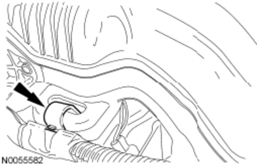
Fig. 382: Locating Block Heater Wiring Harness Retainer From Upper Intake Manifold Courtesy of FORD MOTOR CO.
