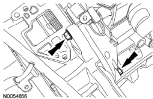
Fig. 123: Locating Engine-To-Transaxle Bolts Courtesy of FORD MOTOR CO.
