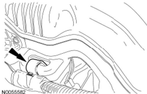
Fig. 1008: Locating Block Heater Wiring Harness Retainer To Upper Intake Manifold Courtesy of FORD MOTOR CO.
