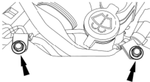
Fig. 138: Locating A/C Tube Retaining Clamp Bolts Courtesy of FORD MOTOR CO.
