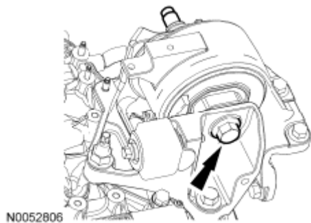
Fig. 112: Locating Transaxle Support Insulator Through Bolt & Nut Courtesy of FORD MOTOR CO.
