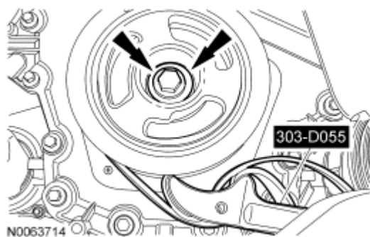
Fig. 24: Installing Crankshaft Pulley Washer & Bolt Using Special Tools (303-D055) Courtesy of FORD MOTOR CO.
