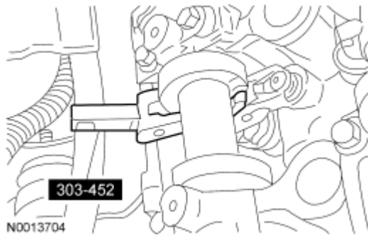
Fig. 636: Using Special Tool (303-452) To Compress Valve Springs Courtesy of FORD MOTOR CO.
