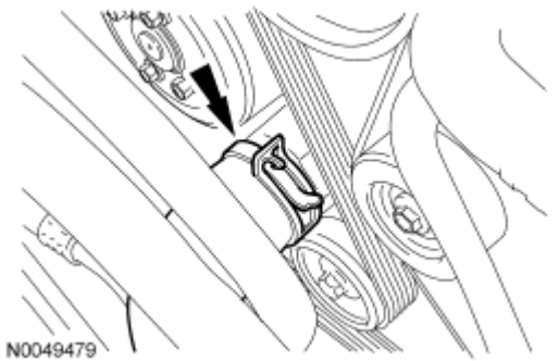
Fig. 751: Disconnecting Coolant Hose From Coolant Pump Courtesy of FORD MOTOR CO.
