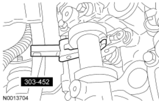
Fig. 117: Using Special Tool (303-452) To Compress Valve Springs Courtesy of FORD MOTOR CO.
