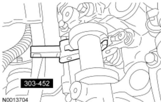
Fig. 106: Using Special Tool (303-452) To Compress Valve Springs Courtesy of FORD MOTOR CO.
