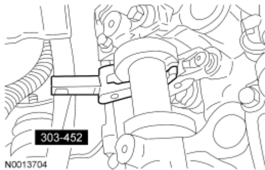
Fig. 520: Using Special Tool (303-452) To Compress Valve Springs Courtesy of FORD MOTOR CO.
