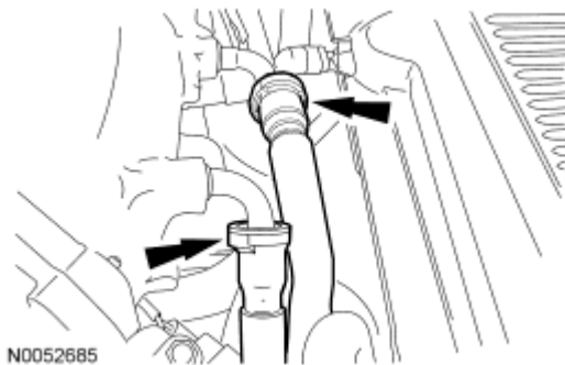
Fig. 298: Disconnecting Evaporative Emissions (EVAP) Tube & Brake Booster Vacuum Supply Tube From Throttle Body (TB) Spacer Courtesy of FORD MOTOR CO.
