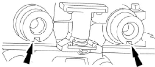
Fig. 91: Identifying Keyways On Camshafts To 6 O'clock Position Courtesy of FORD MOTOR CO.
