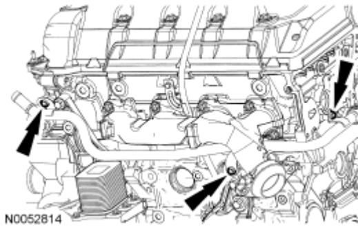
Fig. 657: Identifying Coolant Tube Assembly Bolts Courtesy of FORD MOTOR CO.
