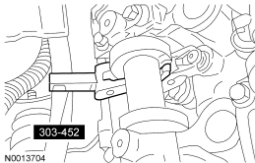
Fig. 111: Using Special Tool (303-452) To Compress Valve Springs Courtesy of FORD MOTOR CO.
