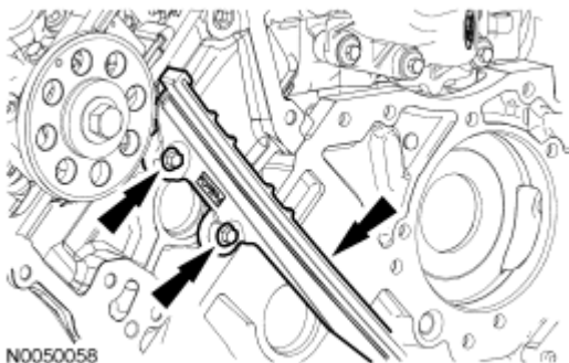
Fig. 58: Locating RH Primary Timing Chain Guide Bolts Courtesy of FORD MOTOR CO.
