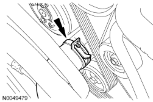
Fig. 296: Disconnecting Coolant Hose From Coolant Pump Courtesy of FORD MOTOR CO.
