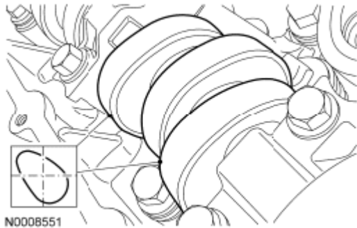
Fig. 181: Identifying Position Of Intake Camshaft Lobes And Exhaust Lobe On No. 1 Cylinder Courtesy of FORD MOTOR CO.
