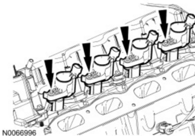
Fig. 591: Locating Ignition Coil Bolts Courtesy of FORD MOTOR CO.
