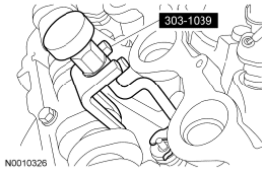
Fig. 411: Removing Valve Spring Retainer Keys Courtesy of FORD MOTOR CO.
