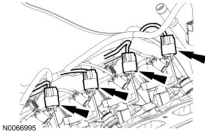
Fig. 11: Locating Ignition Coil Electrical Connectors Courtesy of FORD MOTOR CO.
