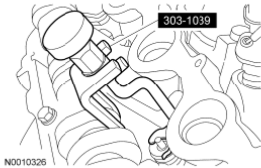
Fig. 189: Removing Valve Spring Retainer Keys Courtesy of FORD MOTOR CO.
