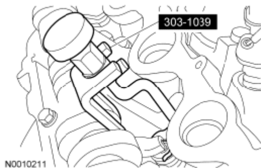
Fig. 172: Removing Camshaft Roller Followers Courtesy of FORD MOTOR CO.
