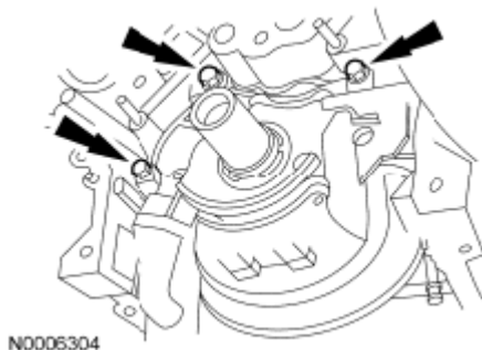
Fig. 435: Locating Oil Pump And Bolts Courtesy of FORD MOTOR CO.
