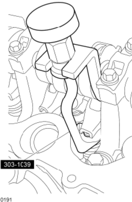
Fig. 107: Removing Valve Spring Compressor (303-1039) On Camshaft Roller Followers Courtesy of FORD MOTOR CO.
