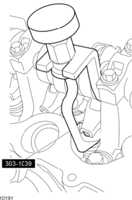
Fig. 163: Installing Valve Spring Compressor Courtesy of FORD MOTOR CO.
