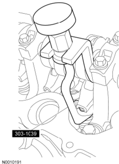
Fig. 121: Identifying Valve Spring Compressor (303-1039) On Camshaft Roller Followers Courtesy of FORD MOTOR CO.
