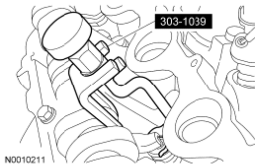
Fig. 191: Installing Camshaft Roller Followers Courtesy of FORD MOTOR CO.
