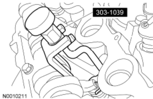
Fig. 187: Installing Camshaft Roller Followers Courtesy of FORD MOTOR CO.
