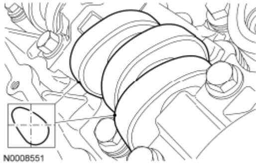
Fig. 128: Identifying Position Of Intake Camshaft Lobes And Exhaust Lobe On No. 1 Cylinder Courtesy of FORD MOTOR CO.
