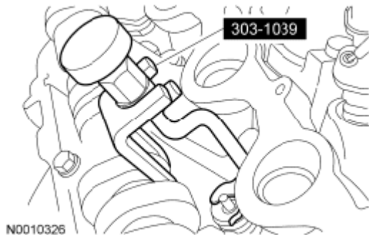
Fig. 190: Removing Valve Spring Retainer Keys Courtesy of FORD MOTOR CO.
