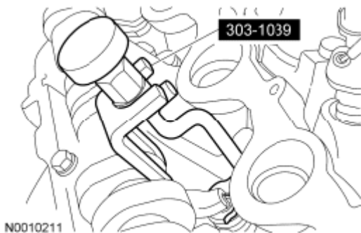
Fig. 182: Installing Camshaft Roller Followers Courtesy of FORD MOTOR CO.
