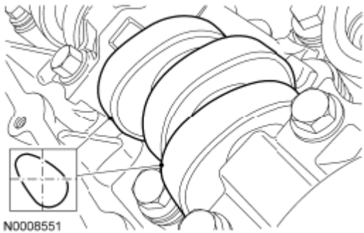
Fig. 314: Identifying Position Of Intake Camshaft Lobes And Exhaust Lobe On No. 1 Cylinder Courtesy of FORD MOTOR CO.
