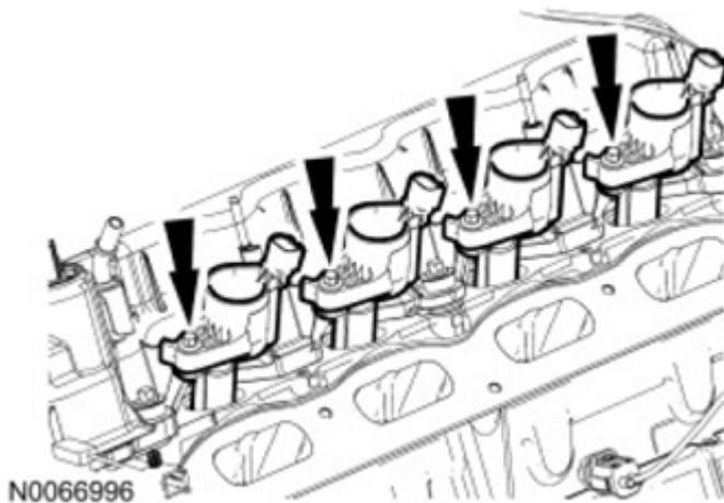
Fig. 358: Locating Ignition Coil Bolts Courtesy of FORD MOTOR CO.
