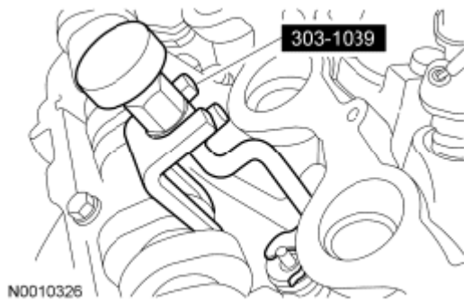
Fig. 193: Removing Valve Spring Retainer Keys Courtesy of FORD MOTOR CO.
