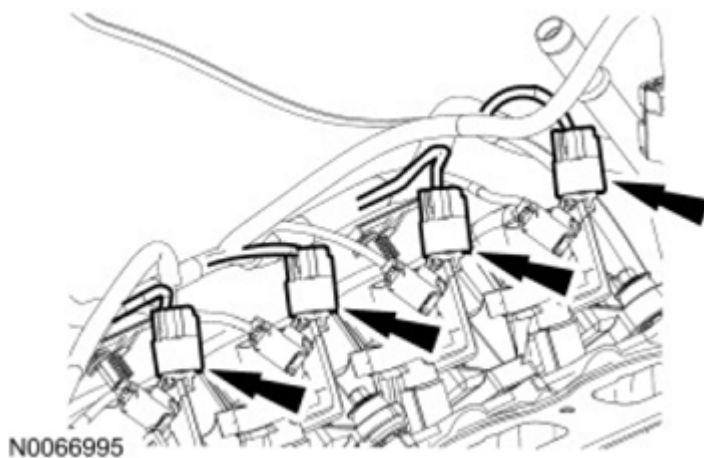
Fig. 13: Locating Ignition Coil Electrical Connectors Courtesy of FORD MOTOR CO.
