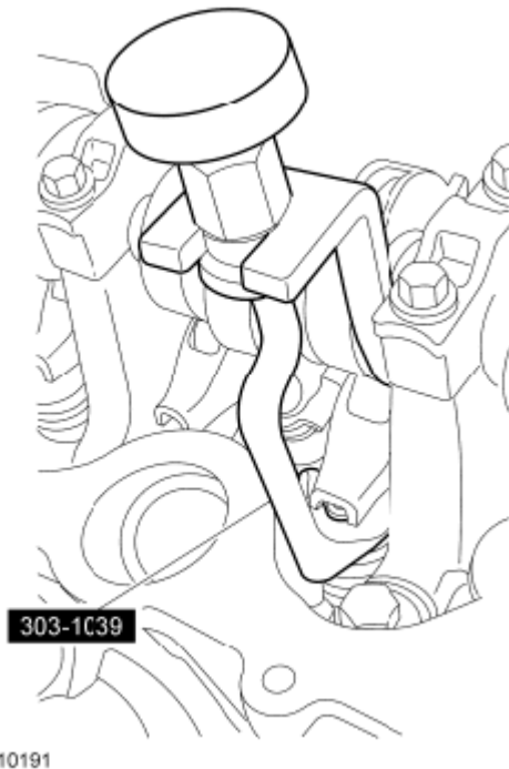
Fig. 462: Installing Camshaft Roller Followers Courtesy of FORD MOTOR CO.
