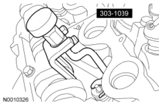
Fig. 195: Installing Valve Spring Retainer Keys Courtesy of FORD MOTOR CO.
