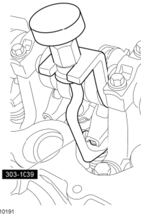
Fig. 67: Removing Designated Camshaft Roller Followers In Previous Step From LH Cylinder Head
