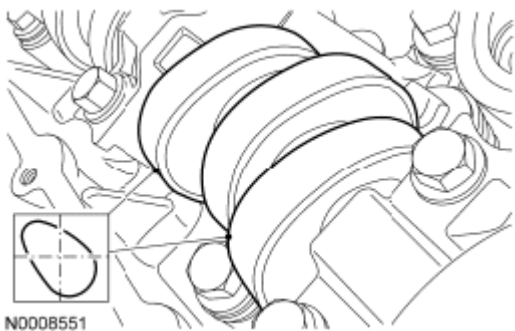
Fig. 170: Identifying Position Of Intake Camshaft Lobes And Exhaust Lobe On No. 1 Cylinder Courtesy of FORD MOTOR CO.
