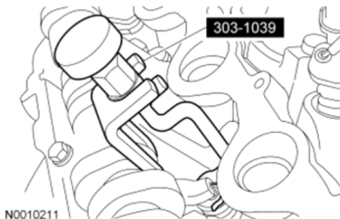
Fig. 217: Removing Camshaft Roller Followers Courtesy of FORD MOTOR CO.
