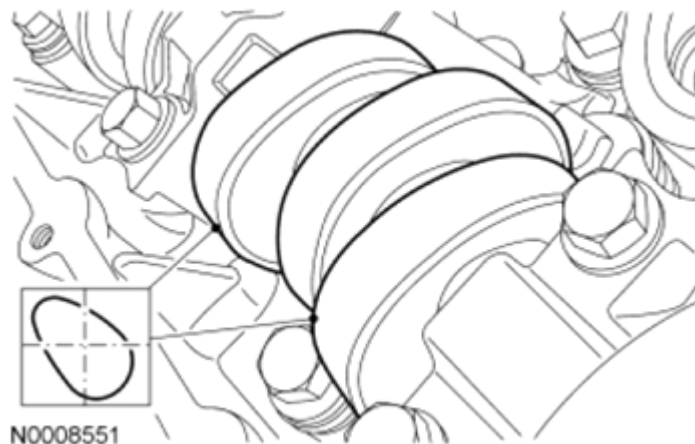
Fig. 401: View Of Intake Camshaft Lobes And Exhaust Lobe On No. 1 Cylinder Courtesy of FORD MOTOR CO.
