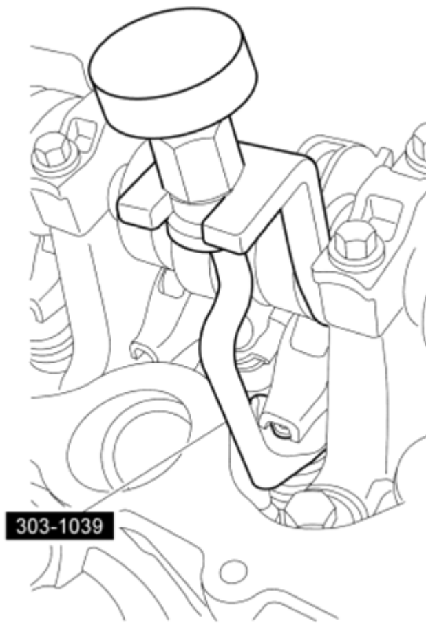
Fig. 126: Using Valve Spring Compressor (303-1039) On Camshaft Roller Followers Courtesy of FORD MOTOR CO.
