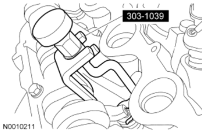
Fig. 213: Removing Camshaft Roller Followers Courtesy of FORD MOTOR CO.
