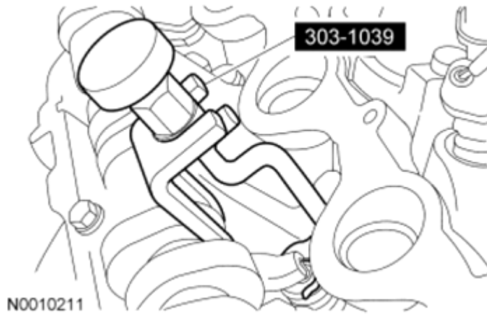
Fig. 343: Removing Camshaft Roller Followers Courtesy of FORD MOTOR CO.
