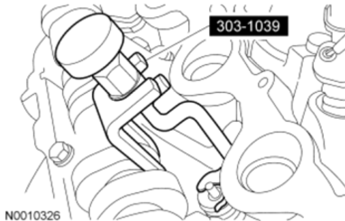
Fig. 433: Removing Valve Spring Retainer Keys Courtesy of FORD MOTOR CO.
