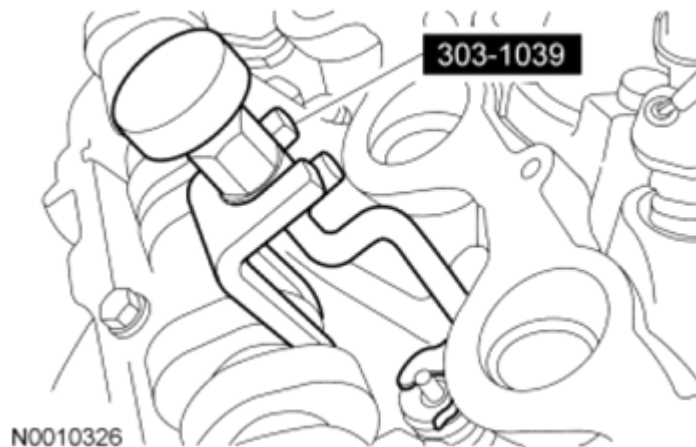
Fig. 220: Installing Valve Spring Retainer Keys Courtesy of FORD MOTOR CO.
