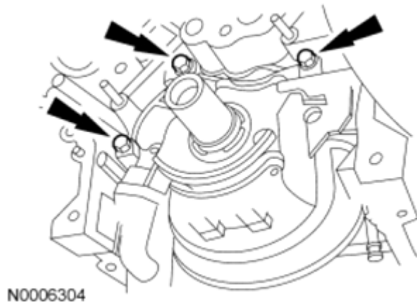
Fig. 424: Locating Oil Pump And Bolts Courtesy of FORD MOTOR CO.
