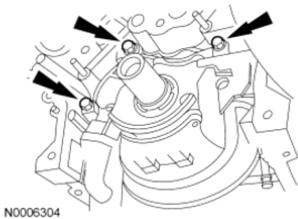
Fig. 253: Locating Oil Pump And Bolts Courtesy of FORD MOTOR CO.
