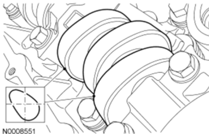
Fig. 341: View Of Intake Camshaft Lobes And Exhaust Lobe On No. 1 Cylinder Courtesy of FORD MOTOR CO.
