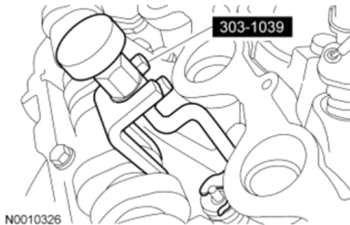
Fig. 218: Removing Valve Spring Retainer Keys Courtesy of FORD MOTOR CO.
