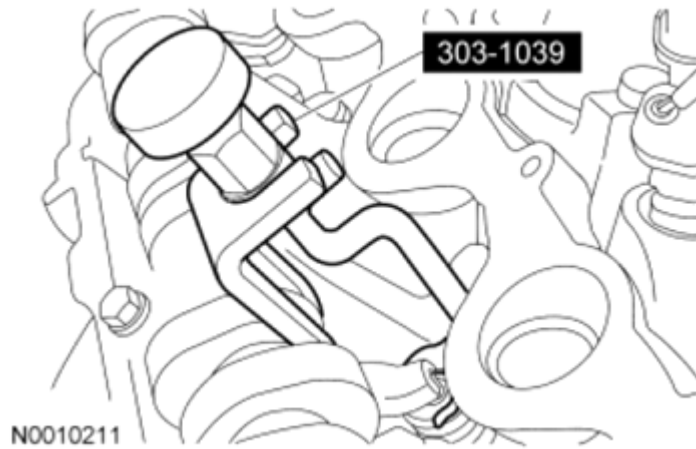
Fig. 216: Installing Camshaft Roller Followers Courtesy of FORD MOTOR CO.
