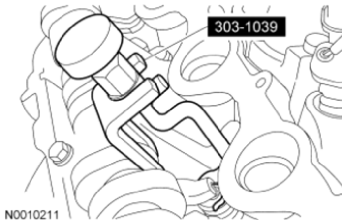
Fig. 212: Installing Camshaft Roller Followers Courtesy of FORD MOTOR CO.
