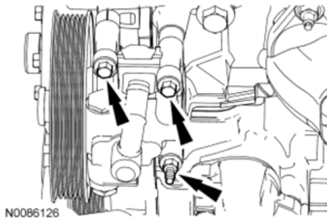
Fig. 62: Locating Power Steering Pump And Bolts Courtesy of FORD MOTOR CO.
