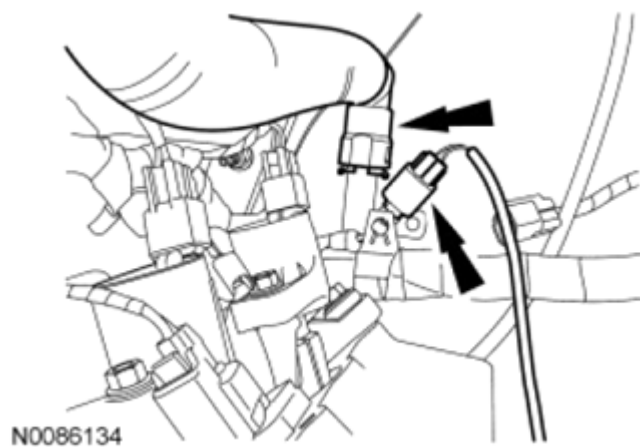
Fig. 311: Locating KS Electrical Connector RH Courtesy of FORD MOTOR CO.
