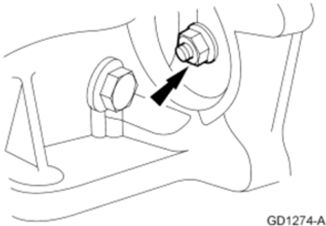
Fig. 290: Locating Torque Converter-To-Flexplate Nuts Courtesy of FORD MOTOR CO.
