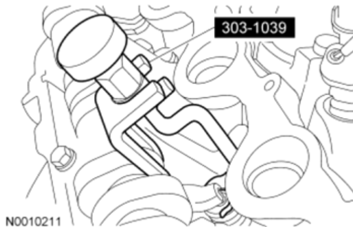
Fig. 84: Removing Camshaft Roller Followers Courtesy of FORD MOTOR CO.
