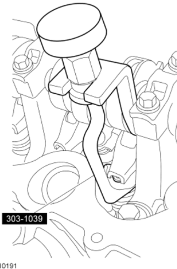
Fig. 119: Using Valve Spring Compressor (303-1039) On Camshaft Roller Followers Courtesy of FORD MOTOR CO.
