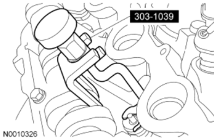
Fig. 214: Removing Valve Spring Retainer Keys Courtesy of FORD MOTOR CO.
