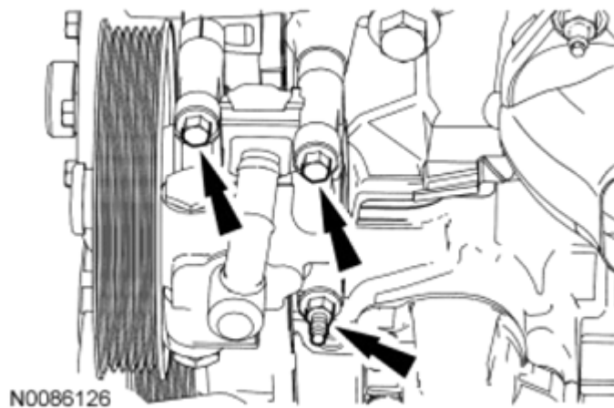
Fig. 307: Locating Power Steering Pump And Bolts Courtesy of FORD MOTOR CO.
