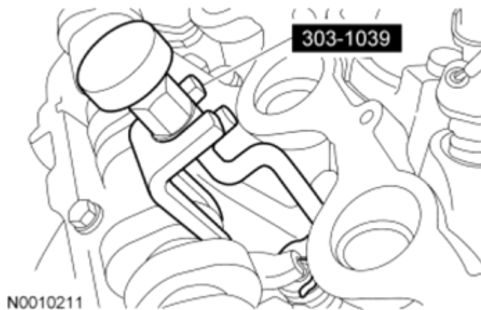
Fig. 221: Installing Camshaft Roller Followers Courtesy of FORD MOTOR CO.
