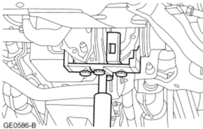
Fig. 233: Positioning Suitable Hydraulic Jack Under Front Axle Courtesy of FORD MOTOR CO.
