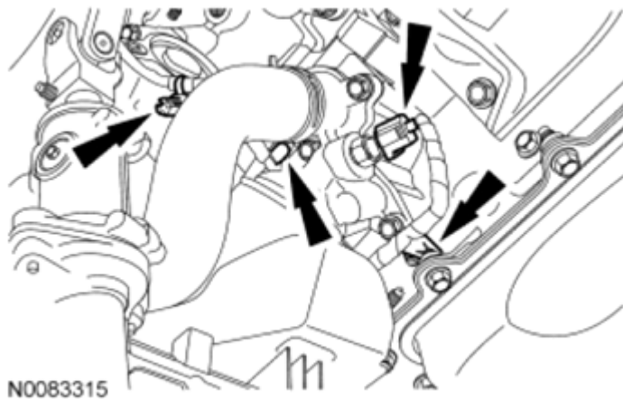
Fig. 298: Locating Engine Oil Pressure (EOP) Switch Electrical Connector And Wiring Harness Retainers Courtesy of FORD MOTOR CO.
