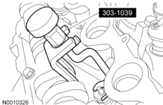
Fig. 431: Removing Valve Spring Retainer Keys Courtesy of FORD MOTOR CO.
