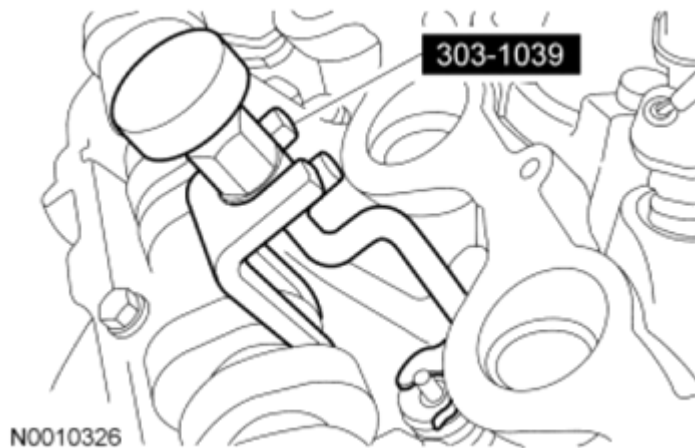
Fig. 215: Installing Valve Spring Retainer Keys Courtesy of FORD MOTOR CO.
