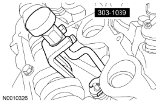
Fig. 431: Identifying Valve Spring Compressor Courtesy of FORD MOTOR CO.
