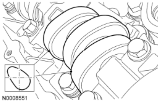
Fig. 200: Identifying Camshaft Lobes Position Courtesy of FORD MOTOR CO.
