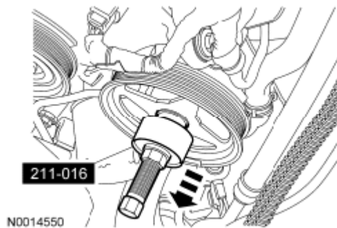
Fig. 306: Removing Power Steering Pump Pulley Courtesy of FORD MOTOR CO.
