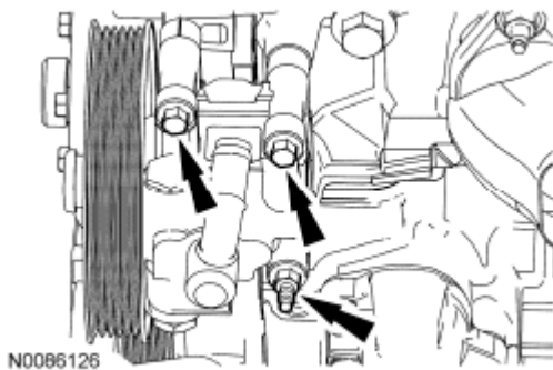
Fig. 553: Locating Power Steering Pump Stud Bolts Courtesy of FORD MOTOR CO.
