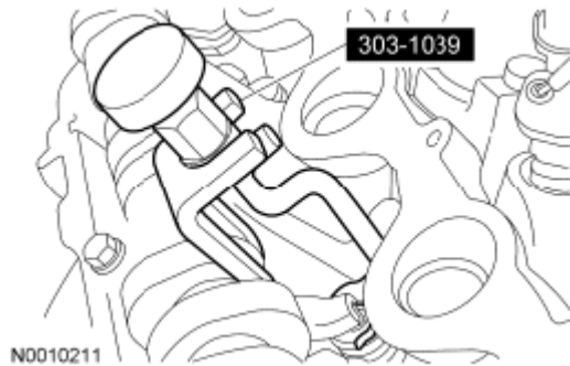
Fig. 403: Identifying Valve Spring Compressor Courtesy of FORD MOTOR CO.
