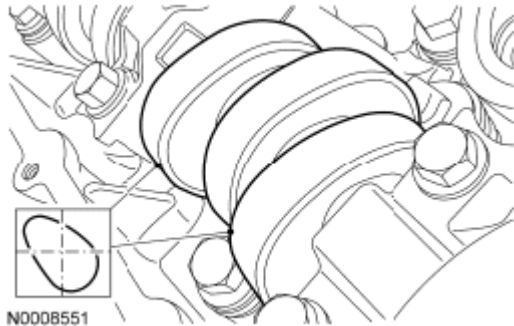
Fig. 147: Identifying Camshaft Lobes Position Courtesy of FORD MOTOR CO.
