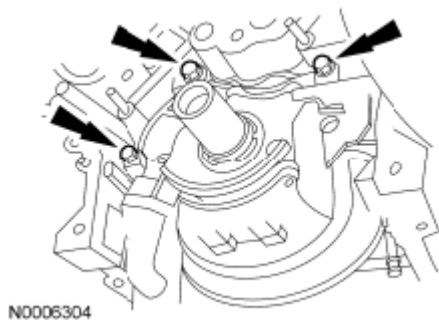
Fig. 458: Locating Oil Pump Bolts Courtesy of FORD MOTOR CO.
