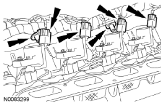
Fig. 316: Locating RH Ignition Coil Electrical Connectors Courtesy of FORD MOTOR CO.
