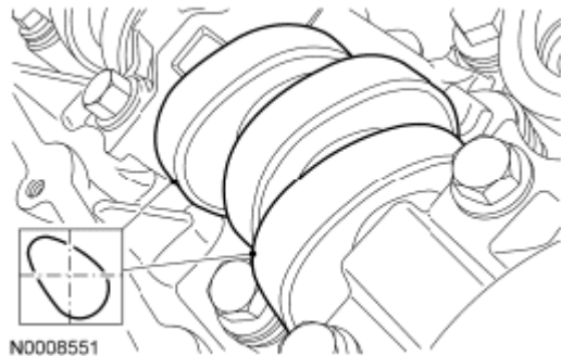
Fig. 189: Identifying Camshaft Lobes Position Courtesy of FORD MOTOR CO.
