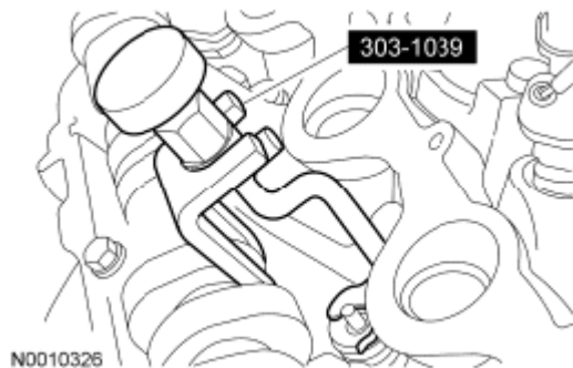
Fig. 215: Identifying Valve Spring Compressor Courtesy of FORD MOTOR CO.
