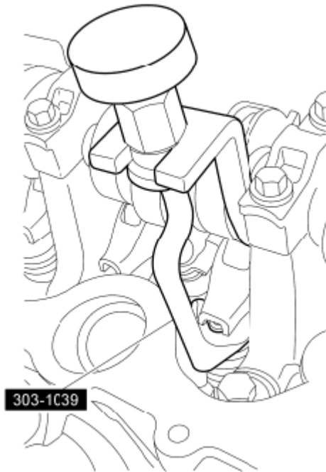
Fig. 172: Identifying Valve Spring Compressor Courtesy of FORD MOTOR CO.
