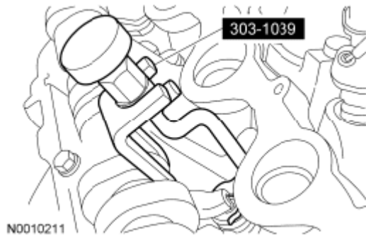
Fig. 84: Identifying Valve Spring Compressor Courtesy of FORD MOTOR CO.
