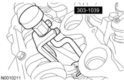
Fig. 212: Identifying Valve Spring Compressor Courtesy of FORD MOTOR CO.
