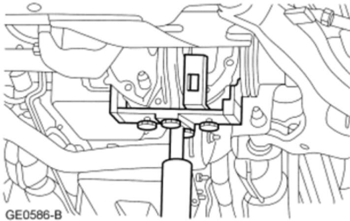
Fig. 247: Supporting Front Axle Carrier Using Hydraulic Jack Courtesy of FORD MOTOR CO.
