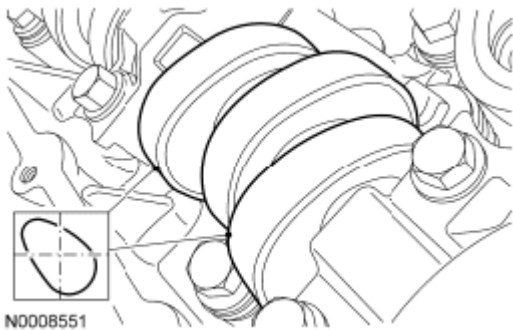
Fig. 82: Identifying Camshaft Lobes Position Courtesy of FORD MOTOR CO.
