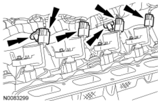
Fig. 547: Locating RH Ignition Coil Electrical Connectors Courtesy of FORD MOTOR CO.
