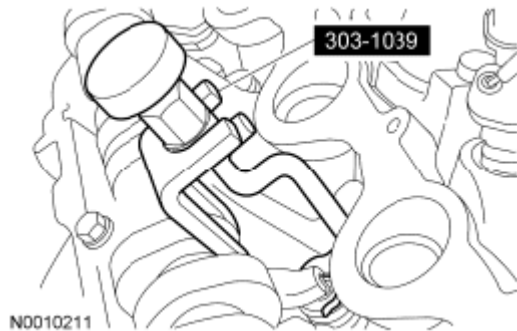
Fig. 343: Identifying Valve Spring Compressor Courtesy of FORD MOTOR CO.
