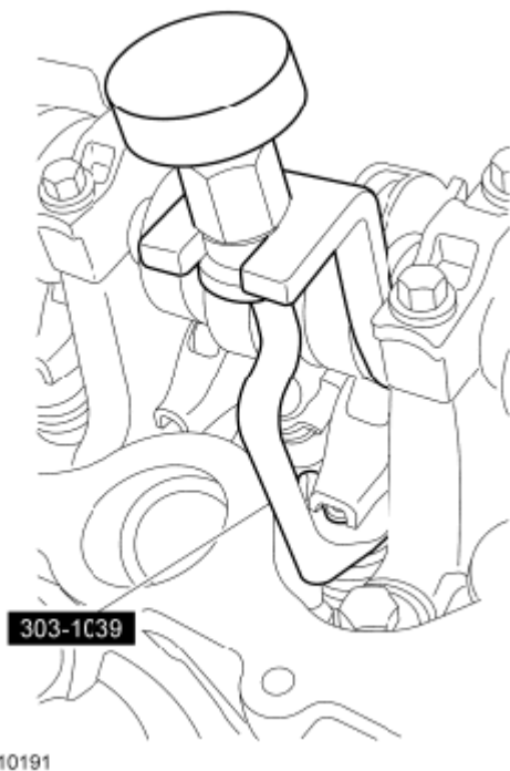
Fig. 182: Identifying Valve Spring Compressor Courtesy of FORD MOTOR CO.
