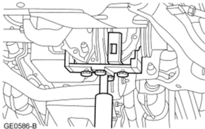
Fig. 233: Supporting Front Axle Using Hydraulic Jack Courtesy of FORD MOTOR CO.
