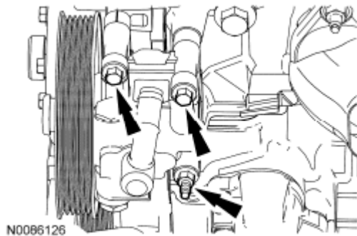
Fig. 307: Locating Power Steering Pump And Reservoir Bolts Courtesy of FORD MOTOR CO.
