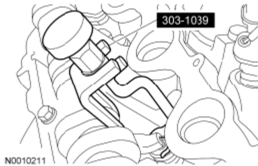
Fig. 221: Identifying Valve Spring Compressor Courtesy of FORD MOTOR CO.
