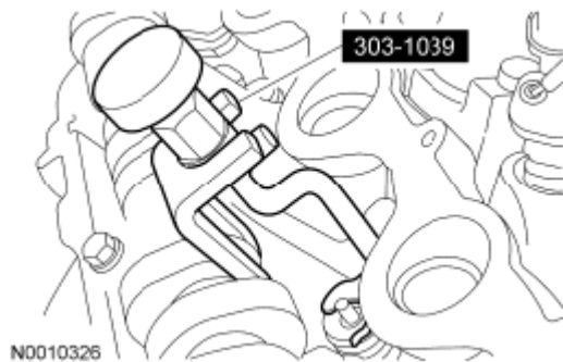
Fig. 220: Identifying Valve Spring Compressor Courtesy of FORD MOTOR CO.
