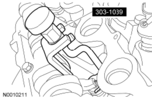
Fig. 149: Identifying Valve Spring Compressor Courtesy of FORD MOTOR CO.
