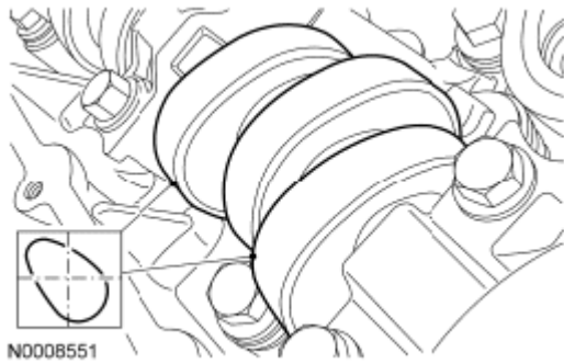
Fig. 401: Identifying Camshaft Lobes Position Courtesy of FORD MOTOR CO.
