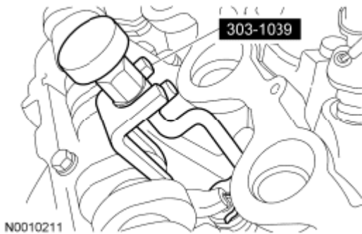
Fig. 163: Identifying Valve Spring Compressor Courtesy of FORD MOTOR CO.
