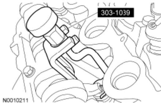
Fig. 211: Identifying Valve Spring Compressor Courtesy of FORD MOTOR CO.
