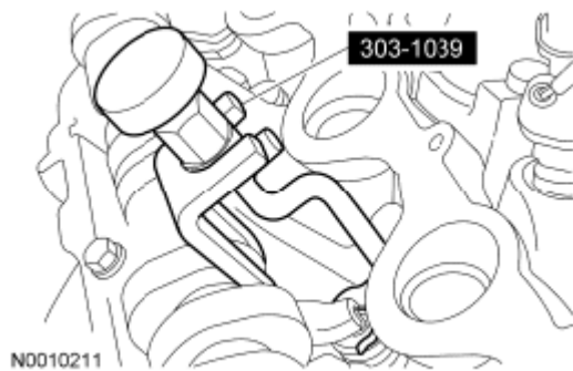
Fig. 213: Identifying Valve Spring Compressor Courtesy of FORD MOTOR CO.
