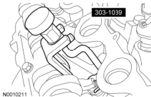
Fig. 217: Identifying Valve Spring Compressor Courtesy of FORD MOTOR CO.
