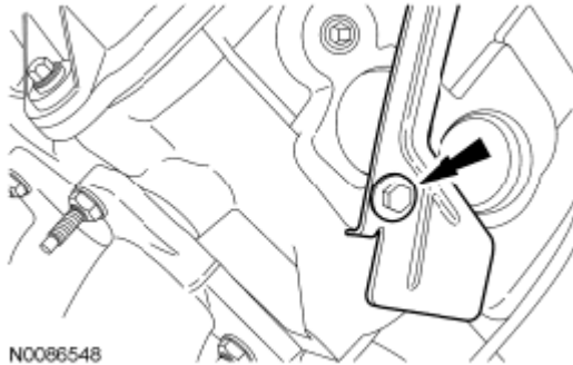
Fig. 611: Locating Intake Manifold Vacuum Tube Support Bracket Bolt Courtesy of FORD MOTOR CO.
