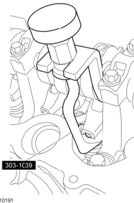
Fig. 405: Identifying Valve Spring Compressor Courtesy of FORD MOTOR CO.
