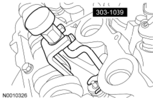
Fig. 218: Identifying Valve Spring Compressor Courtesy of FORD MOTOR CO.
