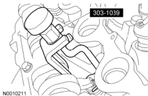
Fig. 216: Identifying Valve Spring Compressor Courtesy of FORD MOTOR CO.
