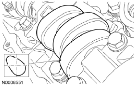
Fig. 341: Identifying Camshaft Lobes Position Courtesy of FORD MOTOR CO.
