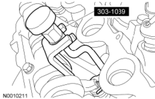
Fig. 360: Removing Camshaft Roller From Cylinder Head RH And Using Valve Spring Compressor Courtesy of FORD MOTOR CO.
