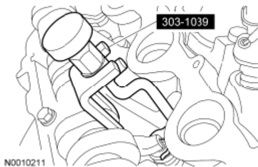
Fig. 216: Removing Camshaft Roller From Cylinder Head RH And Using Valve Spring Compressor
