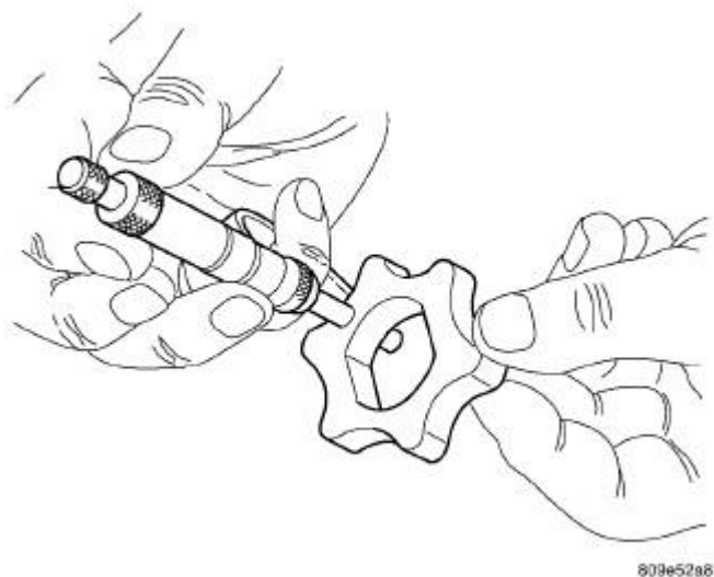
Fig. 288: Measuring Inner Rotor Thickness Courtesy of CHRYSLER GROUP, LLC
