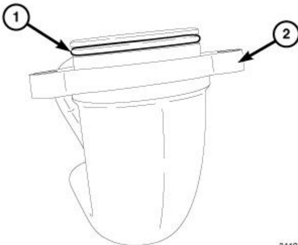
Fig. 341: CAC Air Tube & O-Ring Seal Courtesy of CHRYSLER GROUP, LLC
