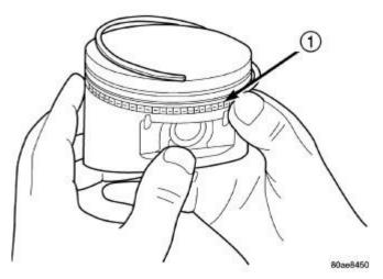
Fig. 203: SIDE RAIL - INSTALLATION Courtesy of CHRYSLER LLC
